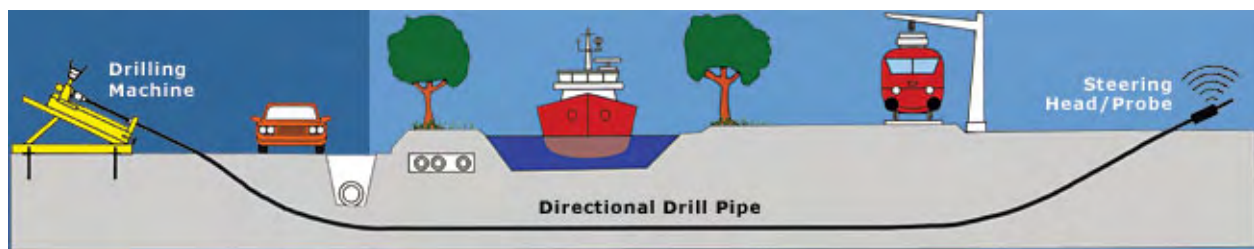
Horizontal Directional Drilling Illustration. Source: http://www.perforator.net/hdd.html
