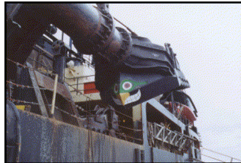
Photo of a turtle deflector attached to a hopper dredge draghead. Source: USACE 2003
