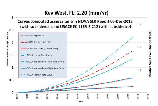
Figure 6: Graphical comparison of the USACE and NOAA Key West sea level rise scenario curves using the USACE sea level rise calculator
