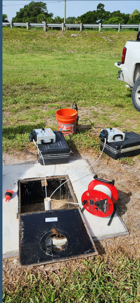
Well being sampled/purged with peristaltic pumps.
