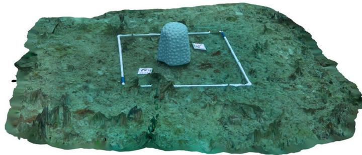
**Figure 3.** 3D model of 3D printed coral colony used to determine model precision in the field photogrammetry methods.
