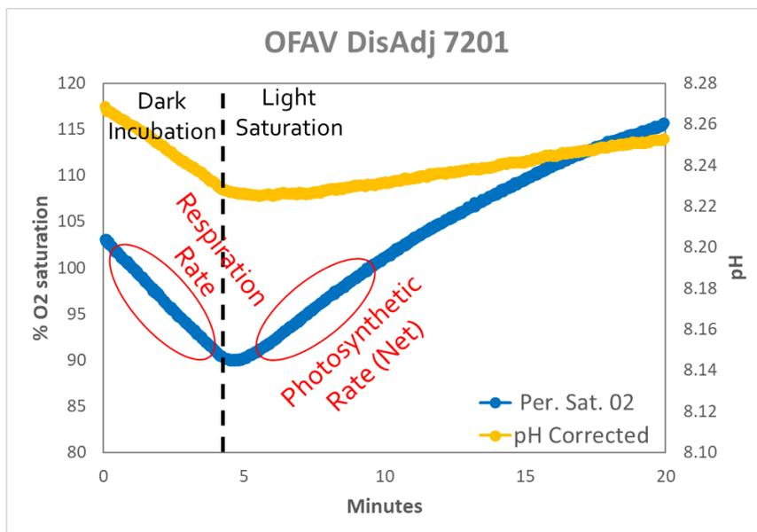
Figure 4. An example sampling run showing the pattern of O<sub>2</sub> saturation and pH through the 4 minute dark incubation and the 16 minute light incubation. Respiration and net photosynthetic rates are calculated from the slopes created by  $\Delta$  O<sub>2</sub> during each incubation period.
