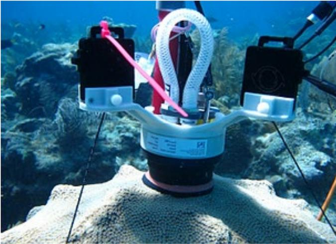
Figure 1. View of CISME chamber head attached to a live coral for metabolic measurements. Photo courtesy of cisme-instruments.com.
