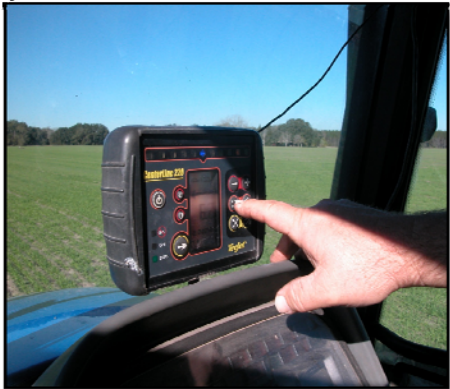
The BMP Implementation Team works with an area farmer to show them the procedures for using a GPS unit in their tractor. This unit is used to more accurately apply fertilizers on the farm.
