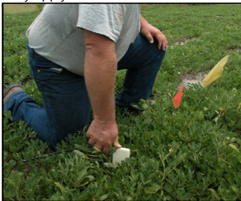
A farmer installs a soil moisture sensor on his farm. This tool allows him to monitor soil moisture continuously to make better informed irrigation decisions.
