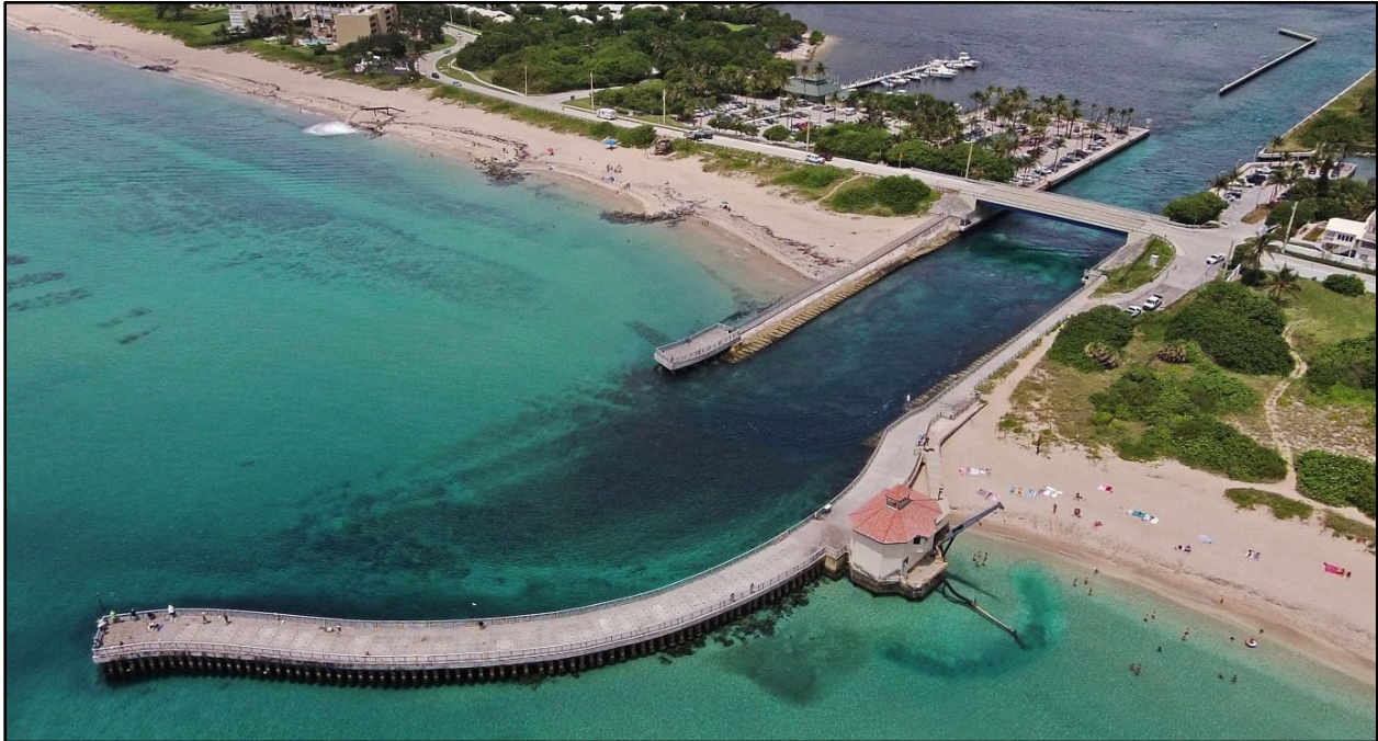
Figure 2. Aerial photograph of South Lake Worth Inlet in 2016, facing southwest. Notable features include the north jetty and sand transfer plant, south jetty, T-head groin field, and A1A bridge. Photo courtesy of Palm Beach County.
