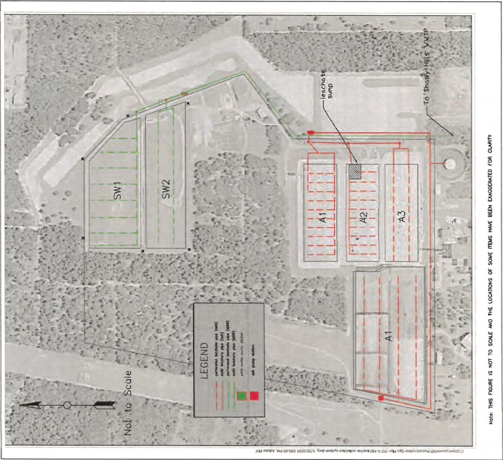
LEACHATE COLLECTION SYSTEM WEST PASCO CLASS I LANDFILL
