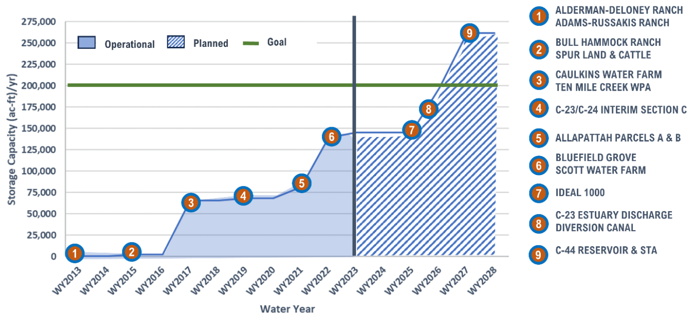
Increasing Project Storage Capacity in the St. Lucie River Watershed
