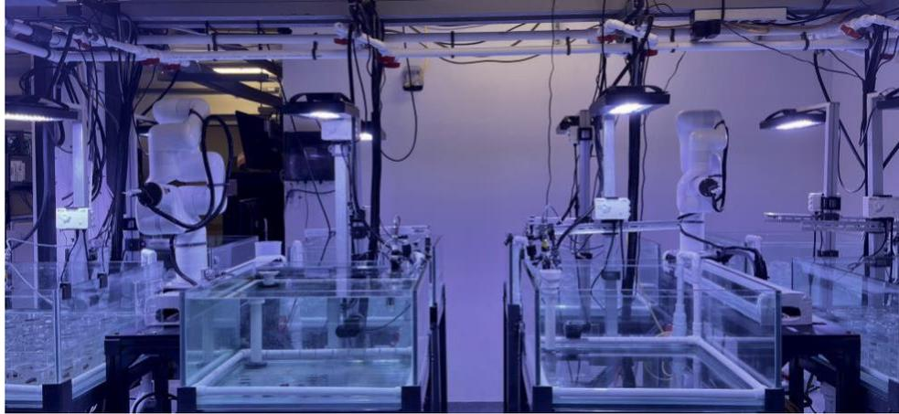
Two robot arms used at the Experimental Reef Lab to dose nutrients and disease into independent coral vessels.
