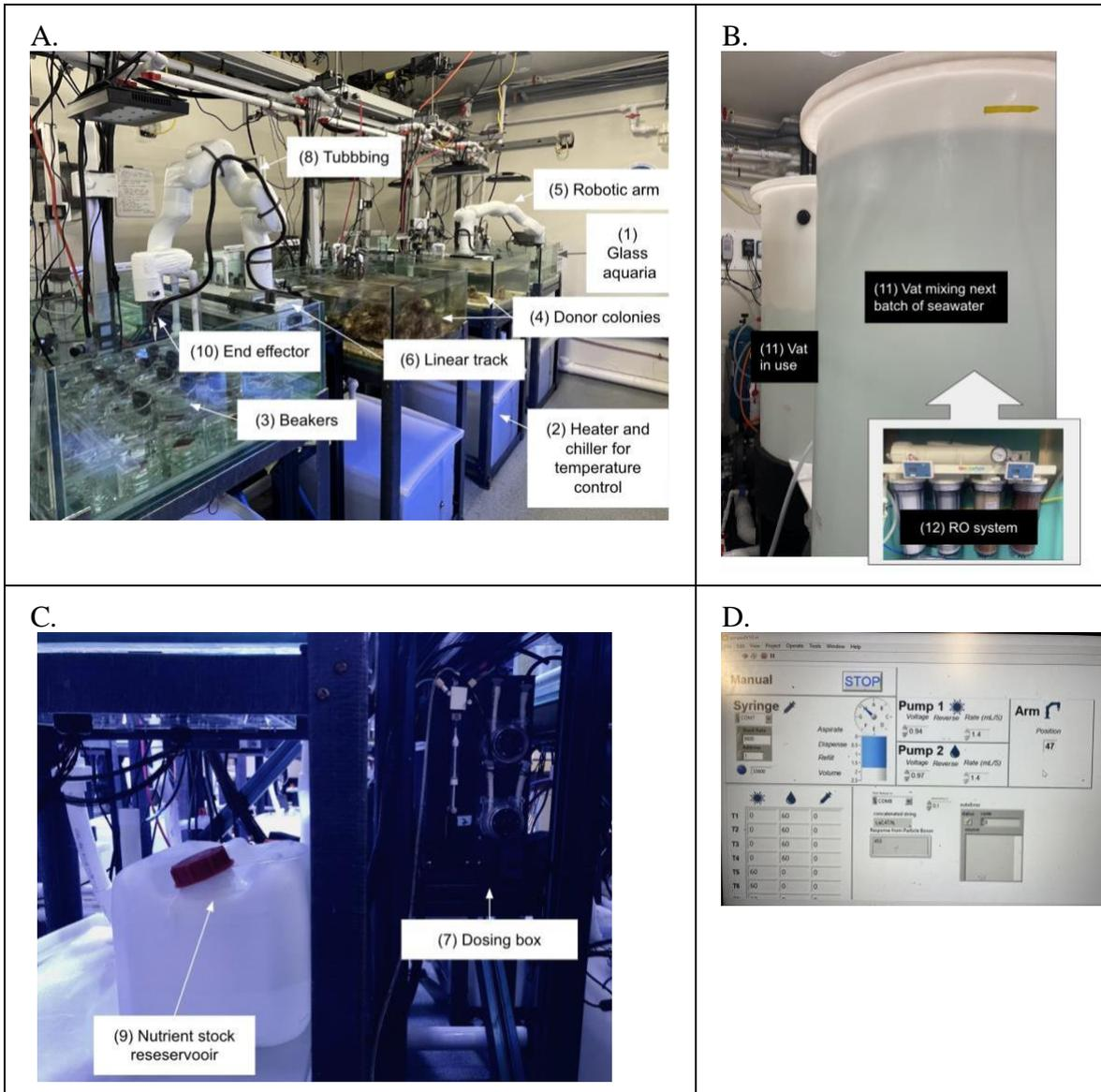
**Figure 1:** STAR system set up in the University of Miami and NOAA Experimental Reef Lab. A. Integrated tanks and arms system, B. Artificial seawater system, C. Dosing box for water and nutrient delivery, and D. LabView graphic interface.
