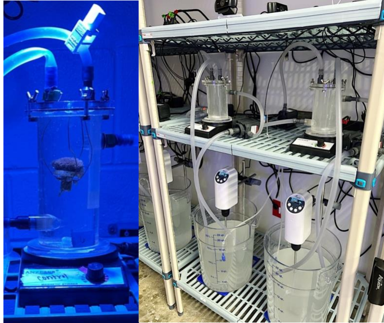
Figure 4. Respirometry setup: A full sump and chamber are set up without coral (Right), and a full chamber is set up with coral exposed to treatment after a flush period (left).
