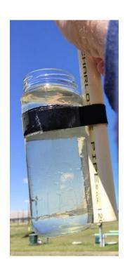
Mature Biofilm → On the pods producing clear, odorless effluent
