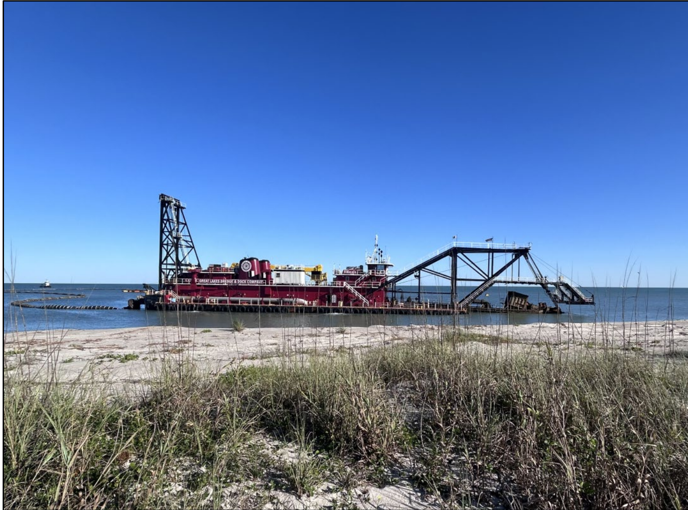
Figure 7. The Great Lakes Dredge & Dock Company (Cutter Suction Dredge, the Illinois) north of Port Canaveral Inlet conducting sand bypassing southward, 2025. Photo courtesy of Mike McGarry (Brevard County) and Dr. Kevin Bodge, P.E., consultant.
