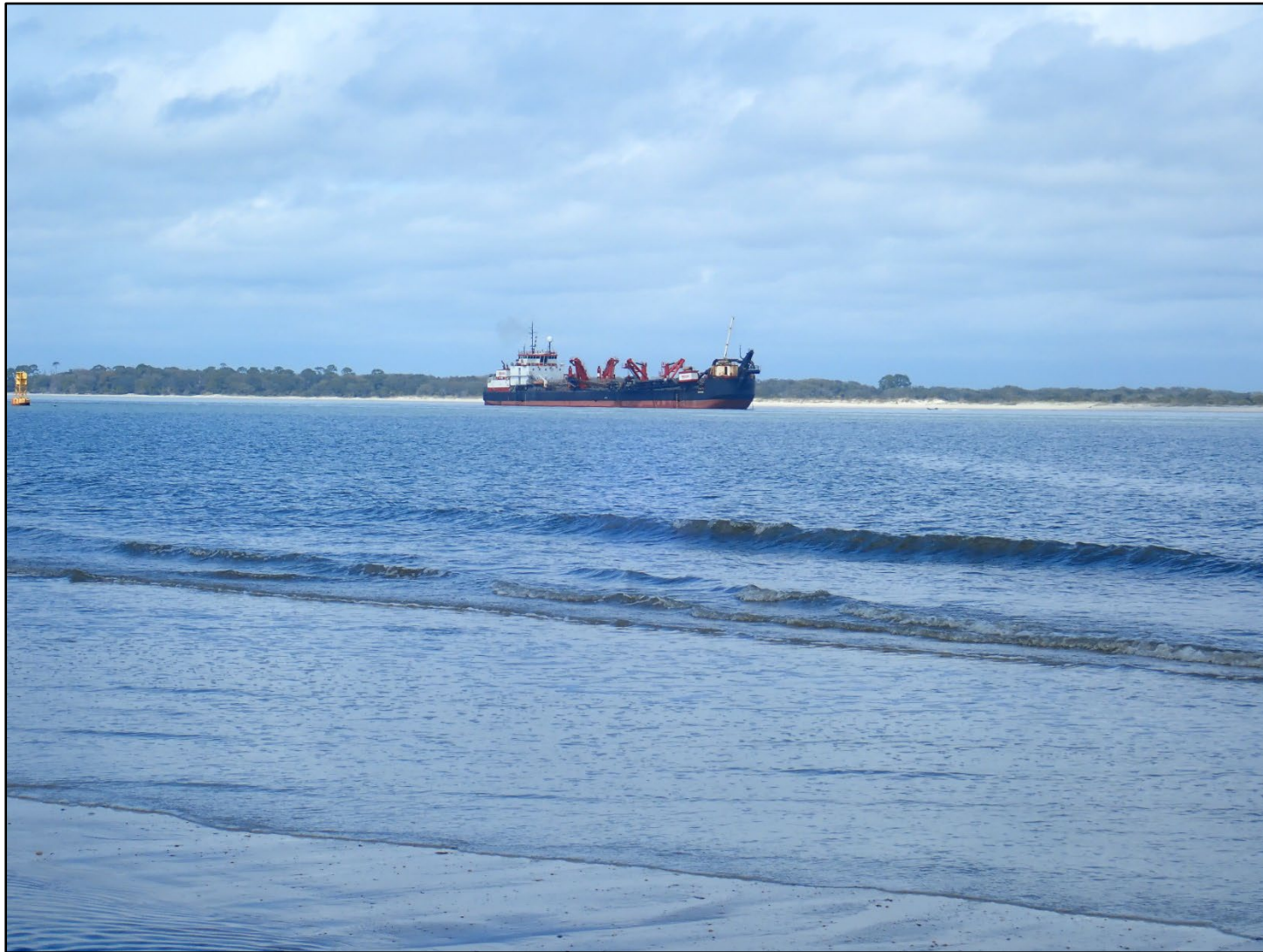
Figure 1: St. Marys River Entrance being dredged by a Manson hopper dredge to bypass material south to Fernandina Beach. Photo by Lindsay Brantley (DEP), March 2022.
