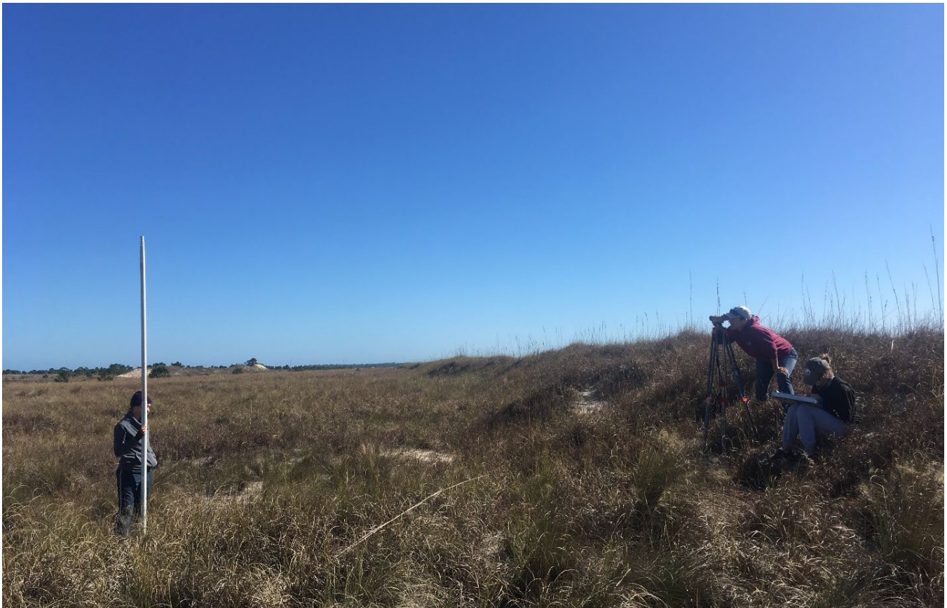
Photo 7 / Reserve staff measuring dune elevation on Little St. George Island to calculate erosion and accretion rates.
