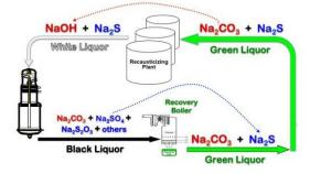
returned to the recovery furnace. The chemicals recovered in the smelt are dissolved in water to make green liquor which is typically reacted with lime to regenerate white liquor. White liquor is used in the pulping process to separate lignin and hemicellulose from the cellulose fiber in wood chips for the production of pulp. Inefficient recovery furnaces require the purchase of raw materials to make up for the lost chemicals.
