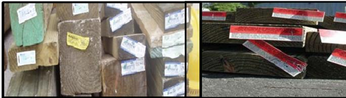
**A1.** Yes. There is a lot of useful information on the labels attached to the end of dimensional wood. Labels identify the type of chemical that was used to treat the wood (CCA, MCQ, MCA, etc.), the level of treatment (pounds of chemical per cubic foot of wood, for example 0.25, 0.40, 0.80, 2.5, etc.) and the location of the treating plant. If the wood has a label then it is probably treated and according to this guidance should be separated out for disposal at a lined disposal facility.
