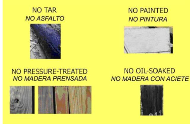
*Explains how to sort wood based on its treatment.*
