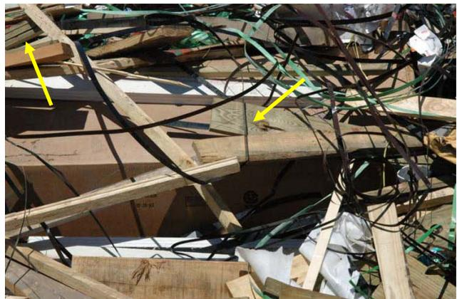
*This load is from a construction company that builds trusses and floor joists. It contains treated wood. Green colored boards are treated. Other boards may be untreated.*
