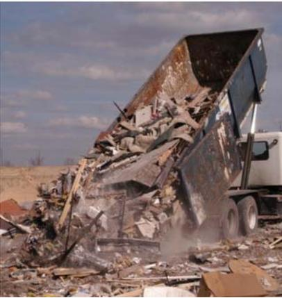
Floor spotters and picking line workers: A trained operator or spotter must inspect the load and pull out larger pieces of treated wood that are listed in the table on page 7. By rule, the MRF must have at least one trained spotter on duty whenever waste is being received. It is recommended that the MRF employ at least one floor spotter per sorting train at the facility. The floor spotter should observe loads as they are tipped onto the tipping floor and
