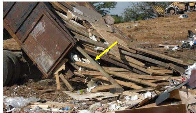
*The green colored pole in the front of this pile is treated. Complete recovery of untreated wood from this pile will likely require testing in addition to visual separation.*
