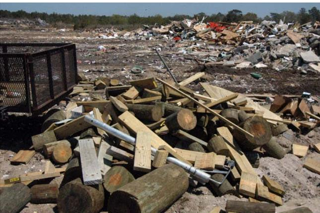
*This load is almost solely CCA-treated wood. It came from a marine construction contractor.*
