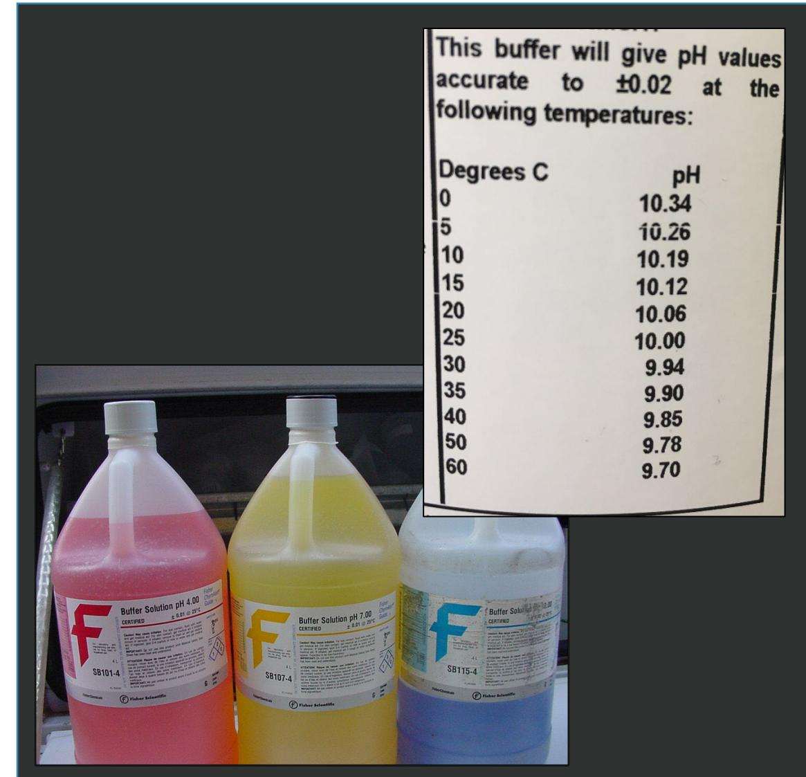
This buffer will give pH values accurate to  $\pm 0.02$  at the following temperatures:
