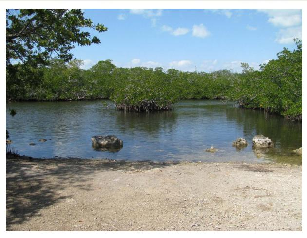
Here is an unimproved soft launch, meaning that no concrete was used. The surface is stable enough for most wheelchairs, and large rocks can be useful for transfers, allowing for better stability and leverage as the user enters or exits the canoe or kayak.
