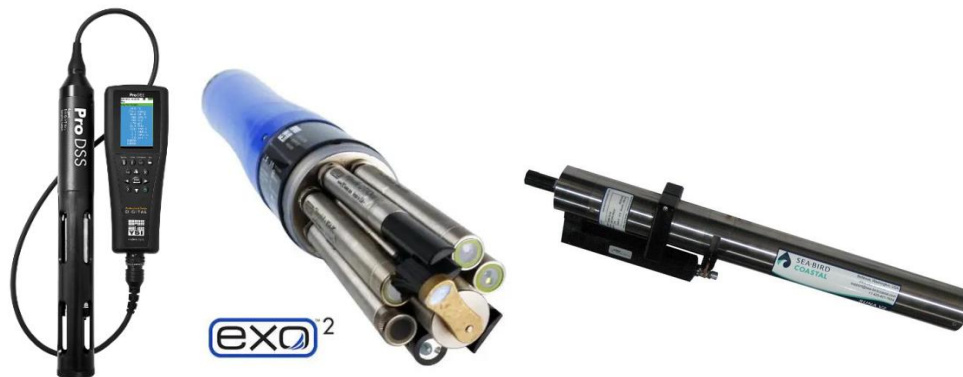
Figure 2. ProDSS, YSI EXO2 and Seabird SUNA nitrogen sensor
