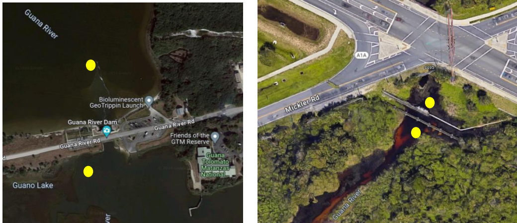
Figure 2. position of the pressure and salinity sensors at the two dams
