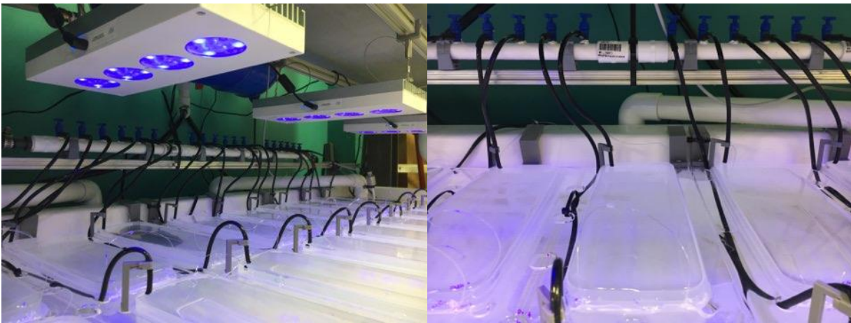
Figure 2. Valve manifolds for delivery of incoming seawater to each experimental aquaria, including 3D printed tubing holders.
