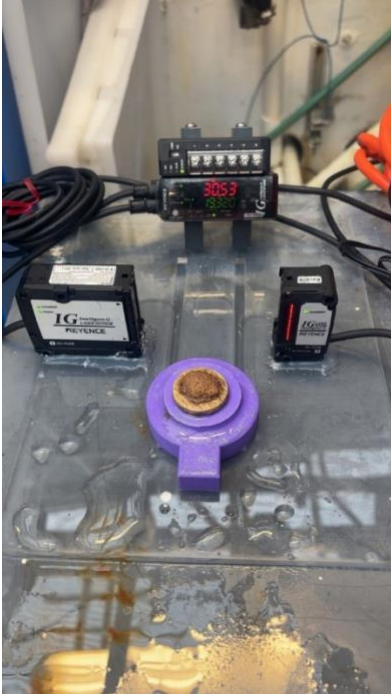
Figure 4. Keyence Intelligent-G Laser Sensor Optical Micrometer used for measuring the vertical growth of the corals.
