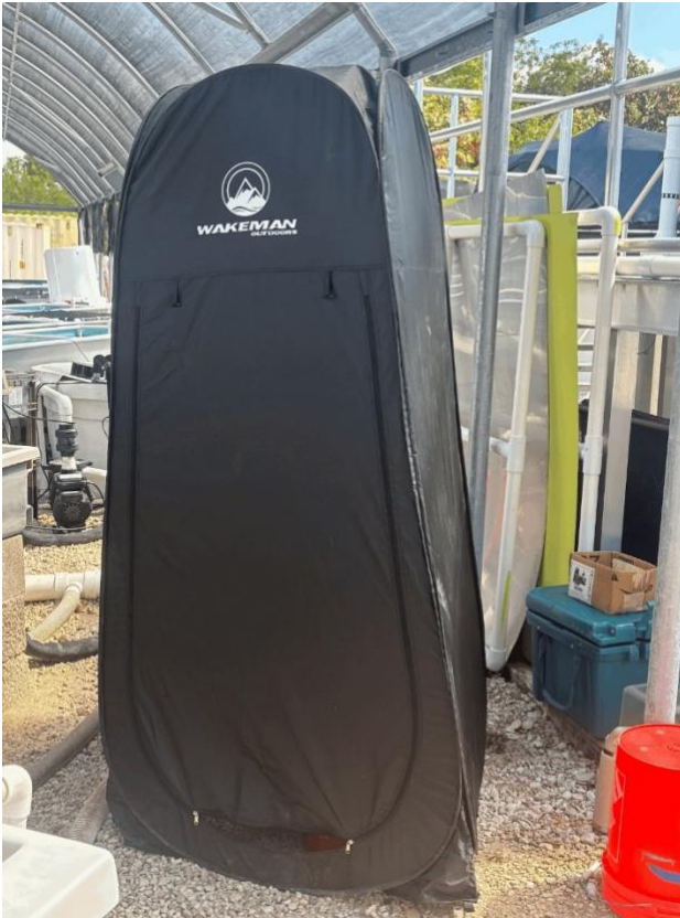
Figure 5. Tent used to provide a dark place for using PAM fluorometer to measure photosynthetic efficiency.
