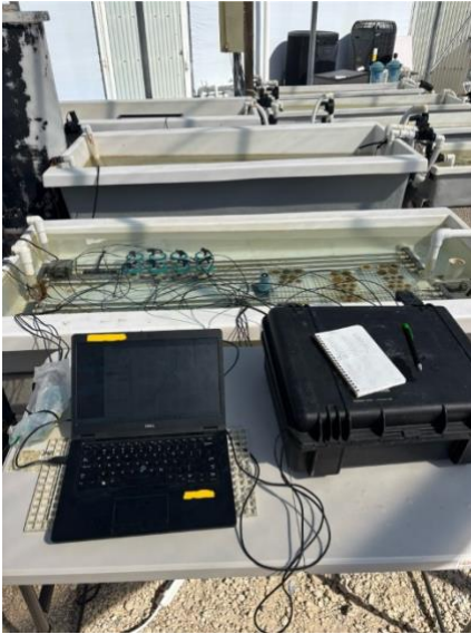
Figure 6. The respirometry setup comprised a laptop computer, a Presens OXY4 oxygen analyzer (in a Pelican case), and glass jars in the raceway tank. Eight corals could be measured at one time. Readings were sent to the computer at 5-second intervals.
