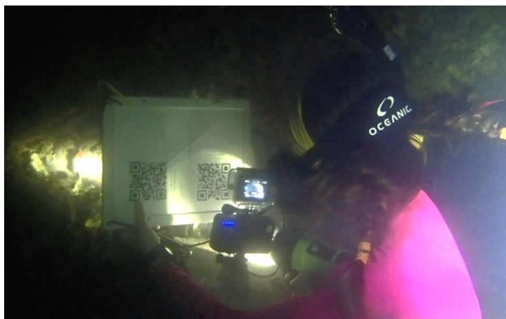
Figure 3. Left: Custom QR code to start a 12-hr time lapse, taking photos every 94 sec. Right: GoPro HERO11 with external battery pack during deployment of experimental time lapse firmware.
