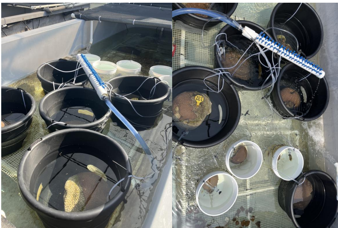
Figure 6. Passive gamete collection apparatus incorporated into land-based aquaculture system at the UM Hatchery, allowing the collection of released gametes from individual broodstock fragments while still maintaining water quality.
