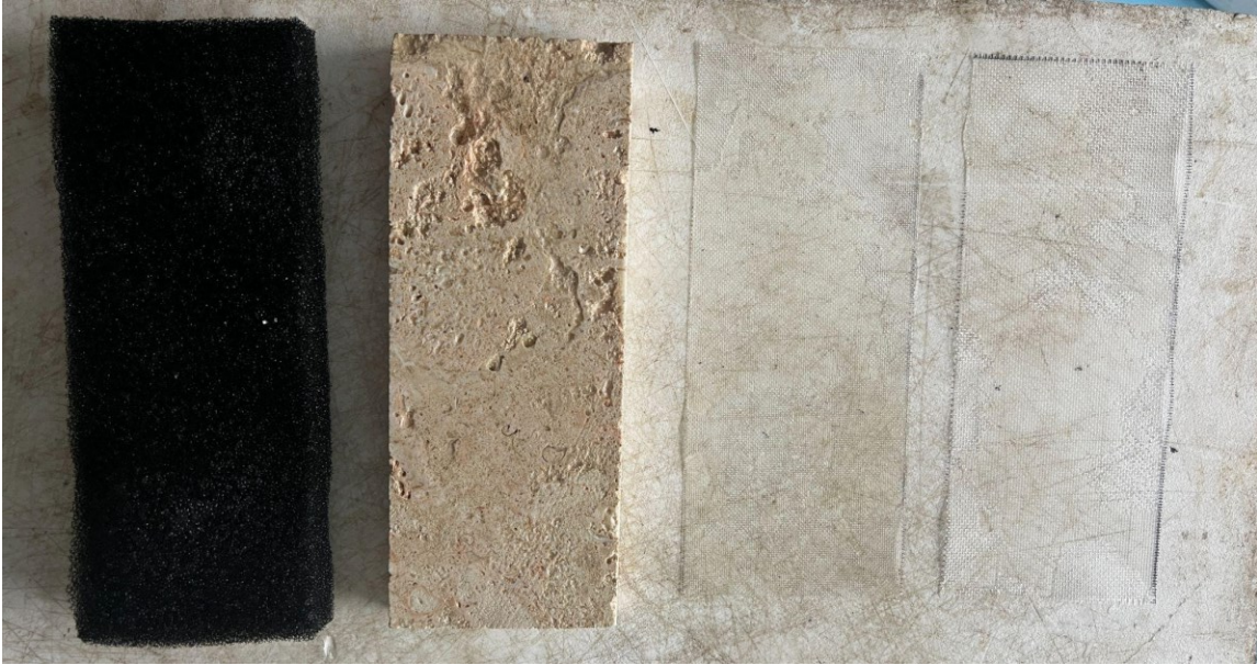
Figure 12. Candidate substrates selected for both Experiment 1 and Experiment 2. Left to Right: Black high density aquaculture filter sponge, cut travertine/limestone tile, 500um nylon mesh, 750um nylon mesh.
