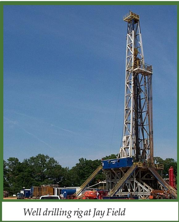
A surface hole is drilled below the base of the underground source of drinking water (typically 1,400 to 2,000 feet deep). Once the specified depth is reached, the drill crew lines the borehole with well casing and cements it in place to prevent wellbore collapse and protect any potential drinking water aquifers. In South Florida, an additional intermediate hole is drilled, cased, and cemented in order to isolate the well from a particularly porous and saline layer known as the “Boulder Zone.”
