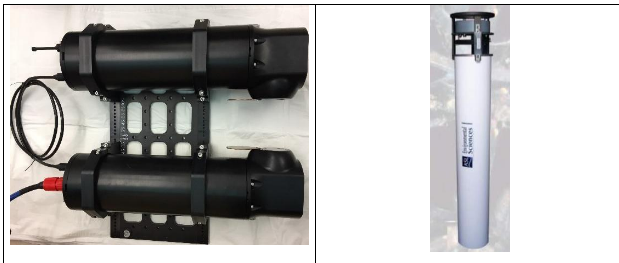
Figure 2D-1: Left: The AUTOHOLO submersible holographic imaging system; Right: the Acoustic Zooplankton Fish Profiler.
