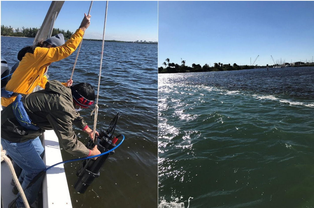
Figure 2D-2: (a) The AUTOHOLO being deployed at one of the stations during the 12/8/20 field effort. (b) Image showing the qualitative difference in turbidity between two distinct water masses during the sampling event.
