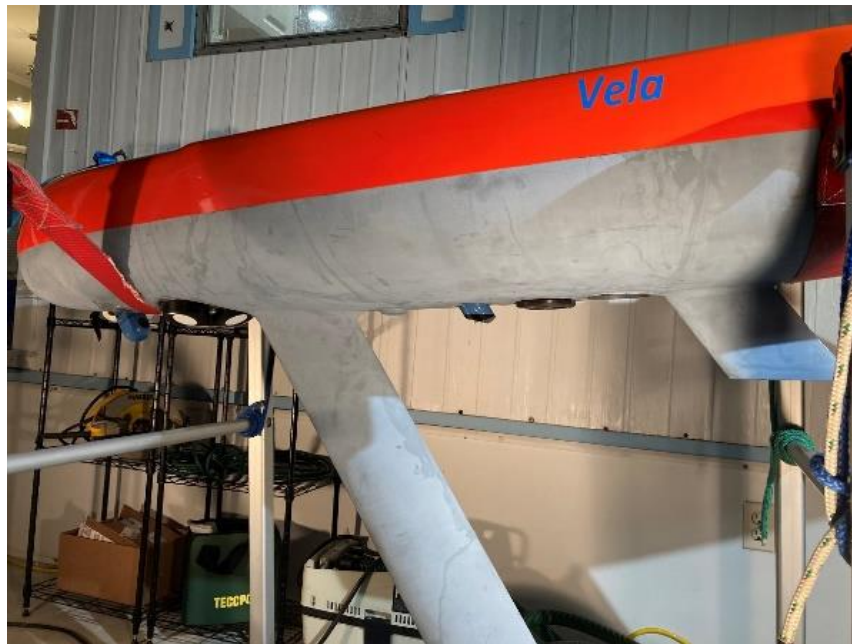
Figure 4-2: Sensors integrated to the ASV hull, left to right: C/T, ADCP, O 2 , CI, and BB3.
