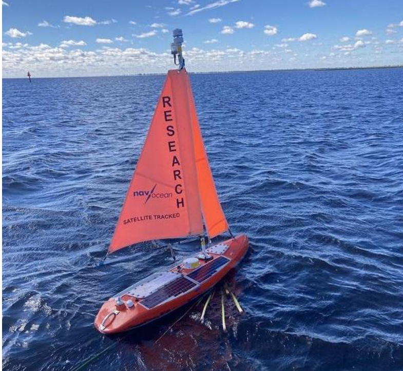
Figure 4-17: Long floating reeds affecting ADCP beams.
