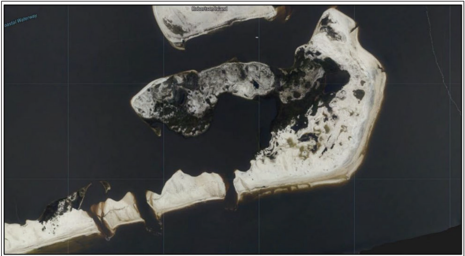
Figure 3. Hurricane Sally breaches through Perdido Key between R60 and R63 near Pensacola Pass (Source: NOAA aerial photography, September 2020).
