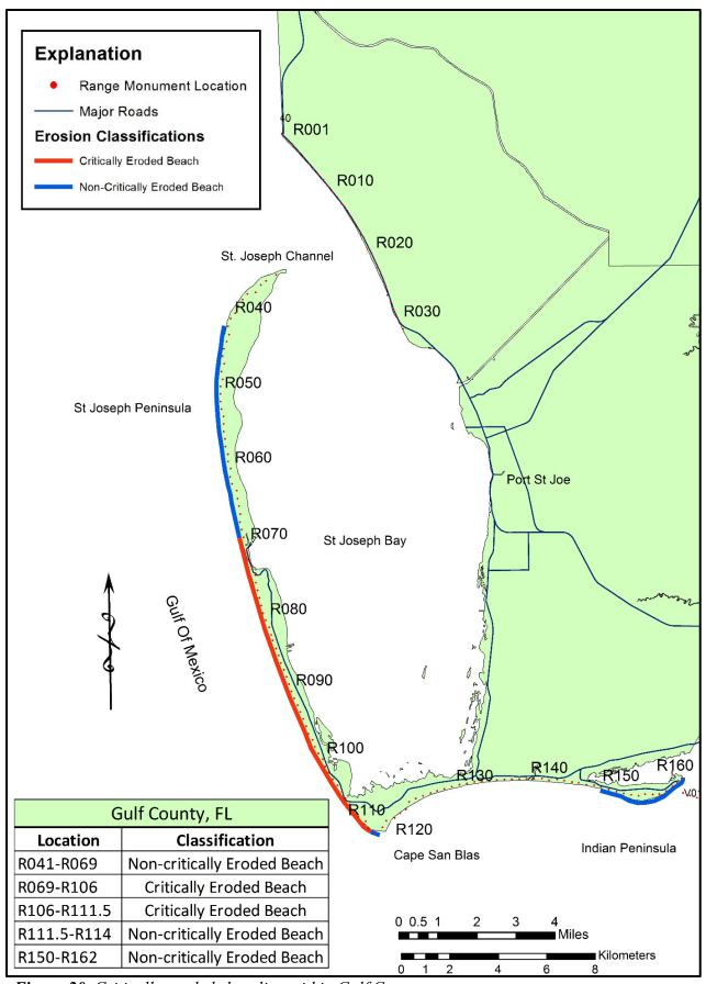
Figure 20. Critically eroded shoreline within Gulf County.
