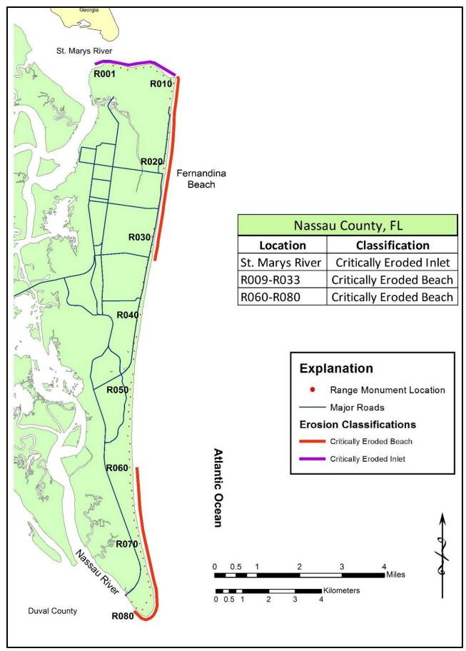
Figure 2. Critically eroded shoreline within Nassau County.
