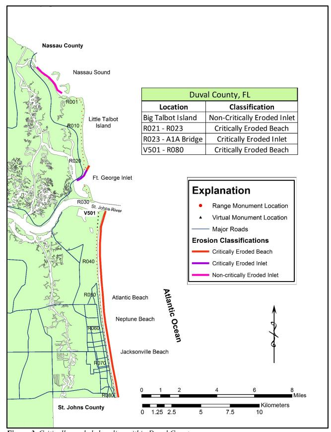
Figure 3. Critically eroded shoreline within Duval County.
