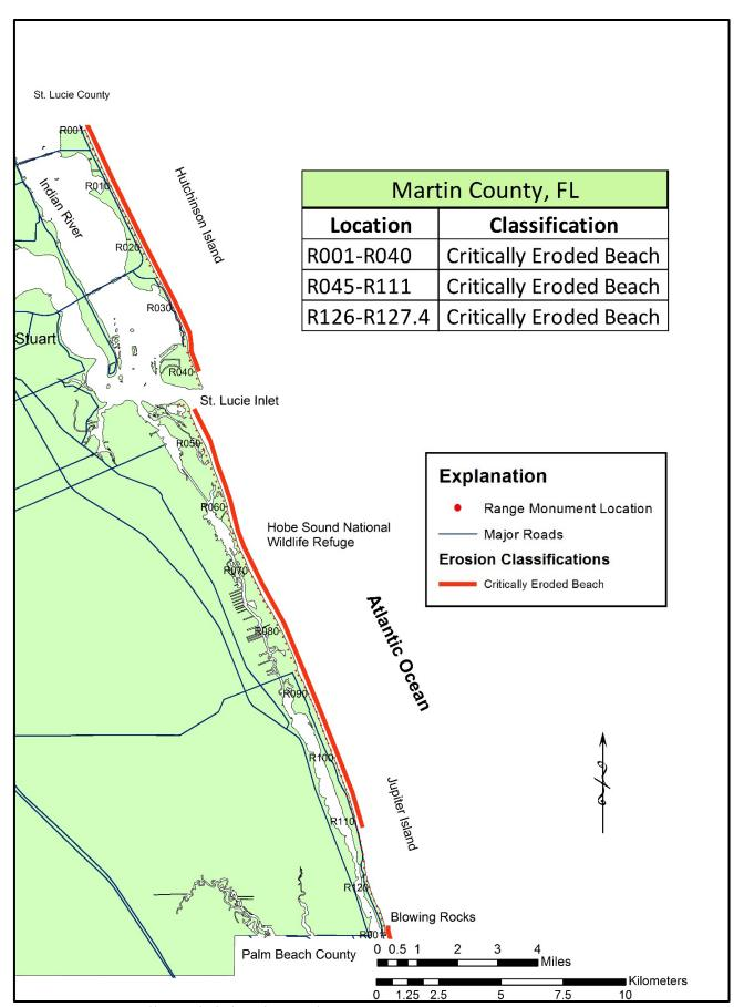
Figure 10. Critically eroded shoreline within Martin County.
