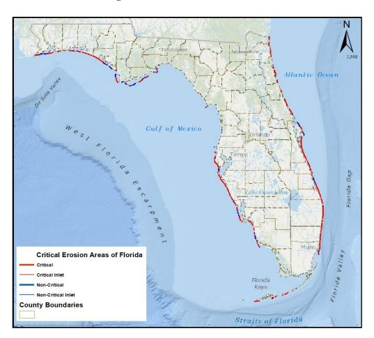
**Figure 1.** Statewide areas of critically and non-critically eroded shoreline [Graphic from <u>ROSSI</u> database]. View an <u>interactive map</u> with aerial imagery showing R monuments and the critical erosion areas.
