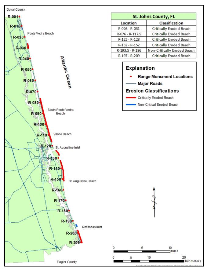
Figure 4. Critically eroded shoreline within St. Johns County.
