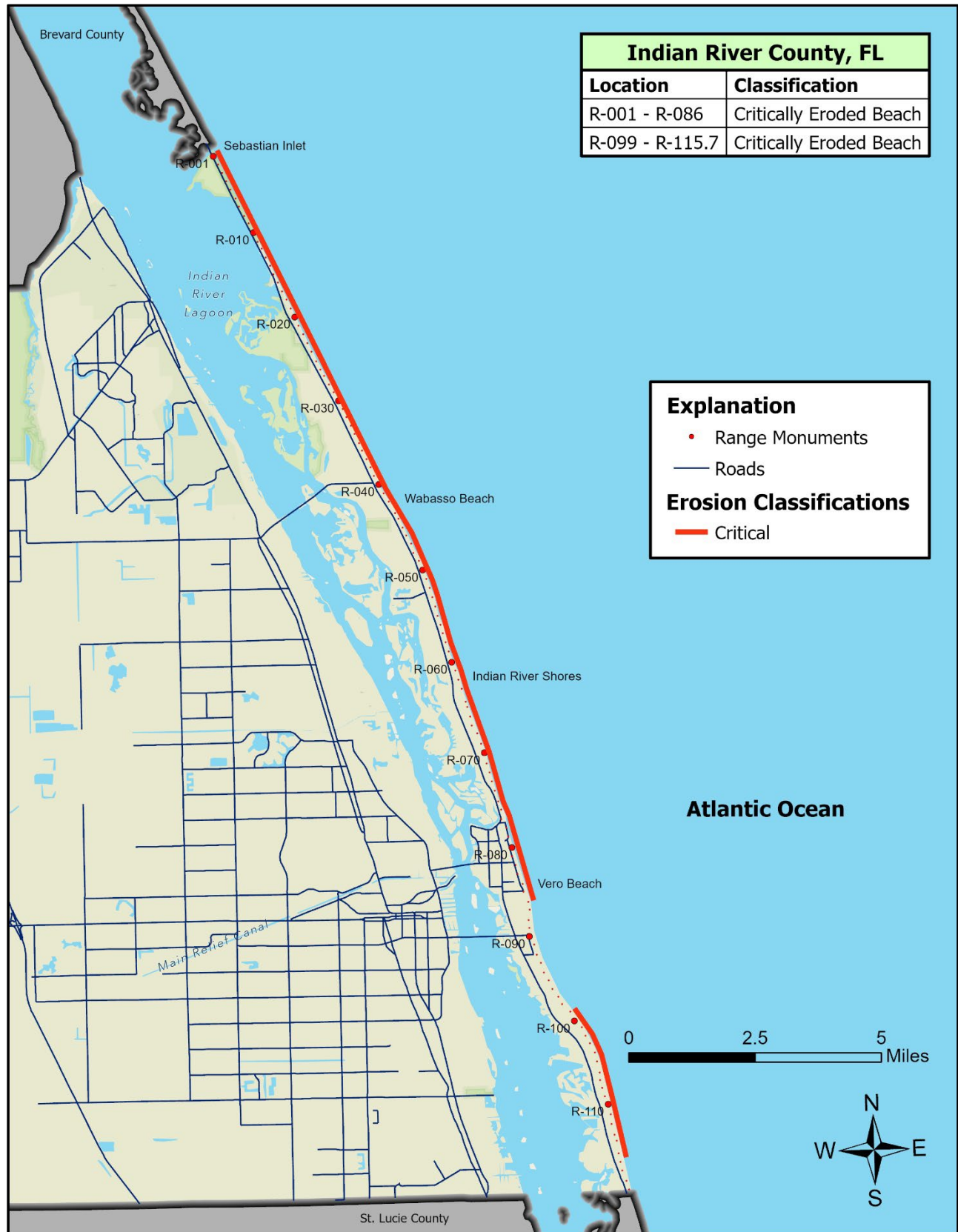
Figure 8. Critically eroded shoreline within Indian River County.
