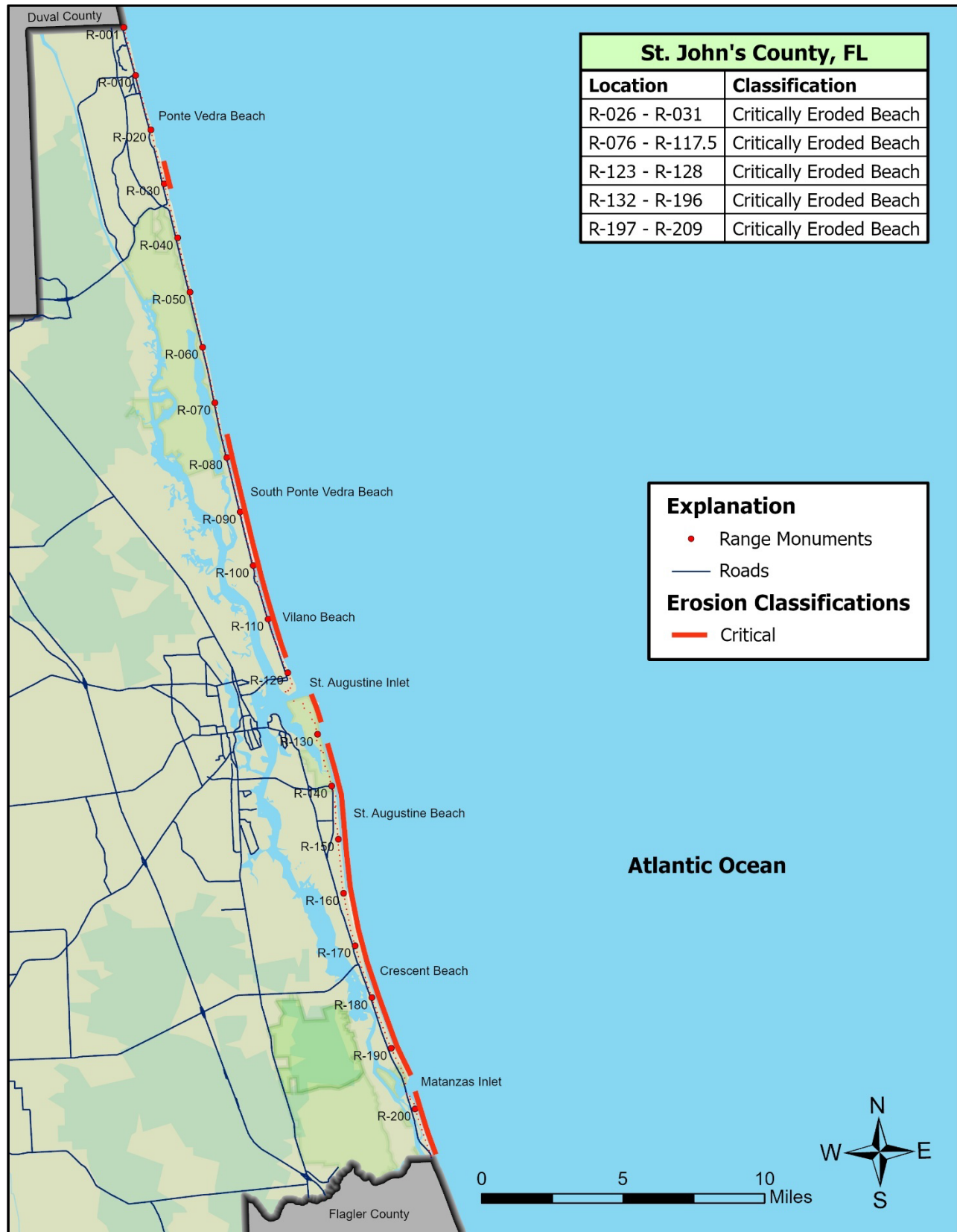
Figure 4. Critically eroded shoreline within St. Johns County.
