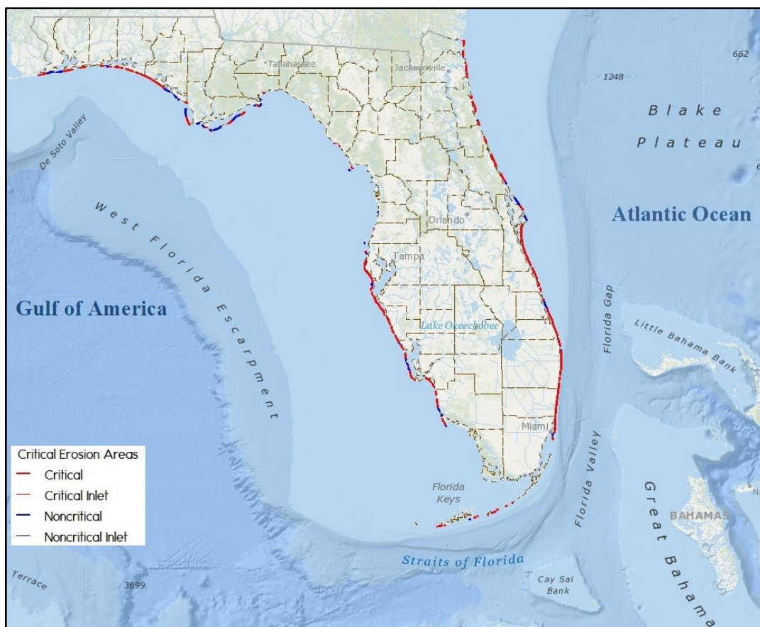
Figure 1. Statewide areas of critically and non-critically eroded shoreline [Graphic from ROSSI database]. View an interactive map with aerial imagery showing R monuments and the critical erosion areas.
