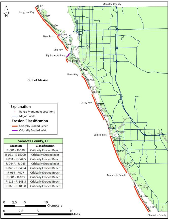
Figure 29. Critically eroded shoreline within Sarasota County.
