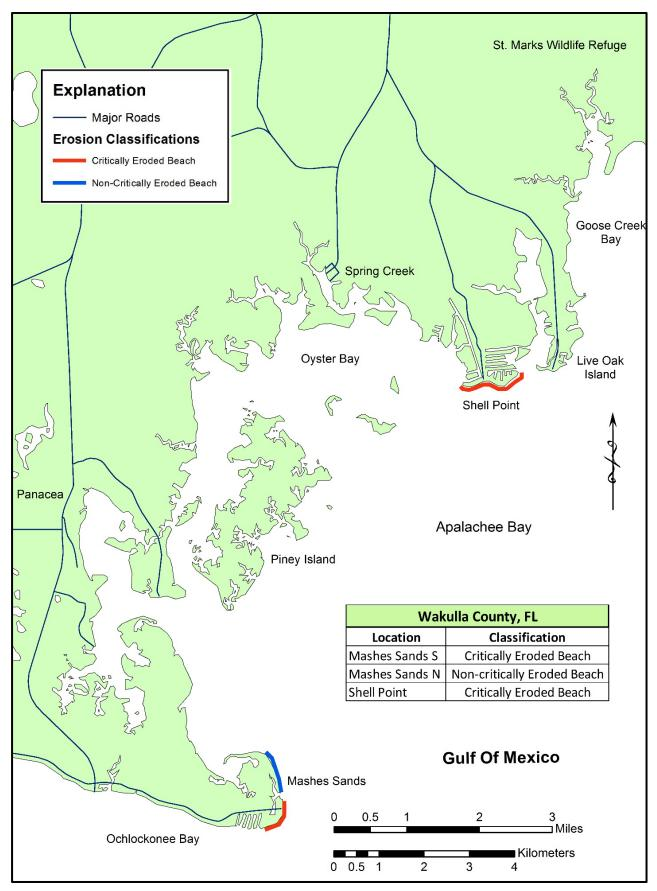
Figure 22. Critically eroded shoreline within Wakulla County.
