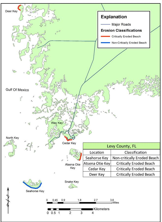
Figure 24. Critically eroded shoreline within Levy County.
