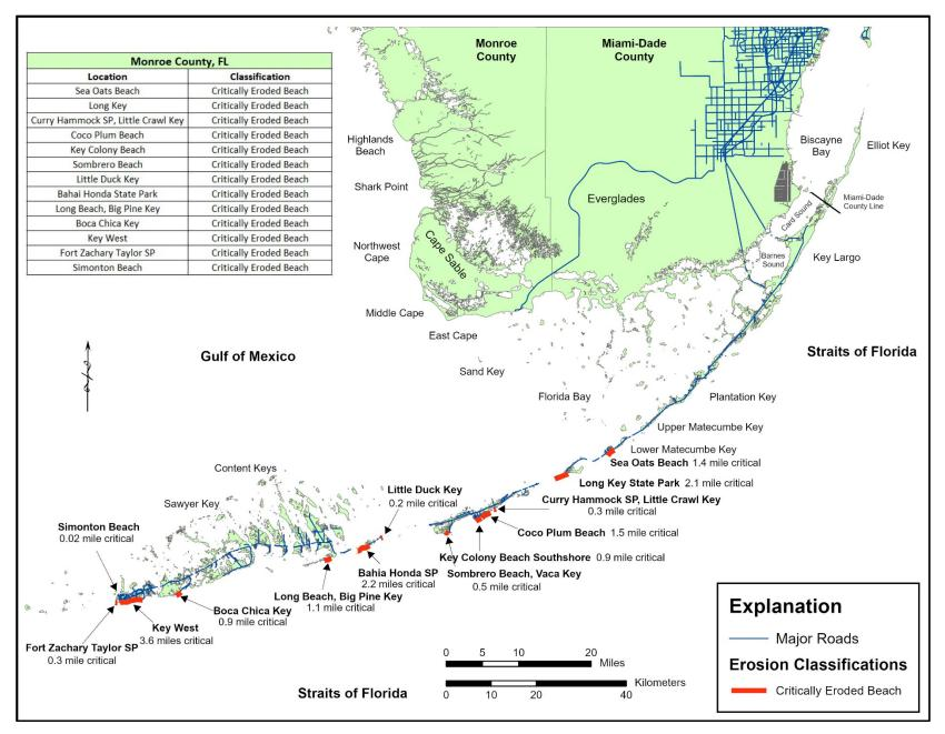
*Figure 14. Critically eroded shoreline within Monroe County – Florida Keys, see <u>Map Direct</u> to zoom into the Florida Keys.*
