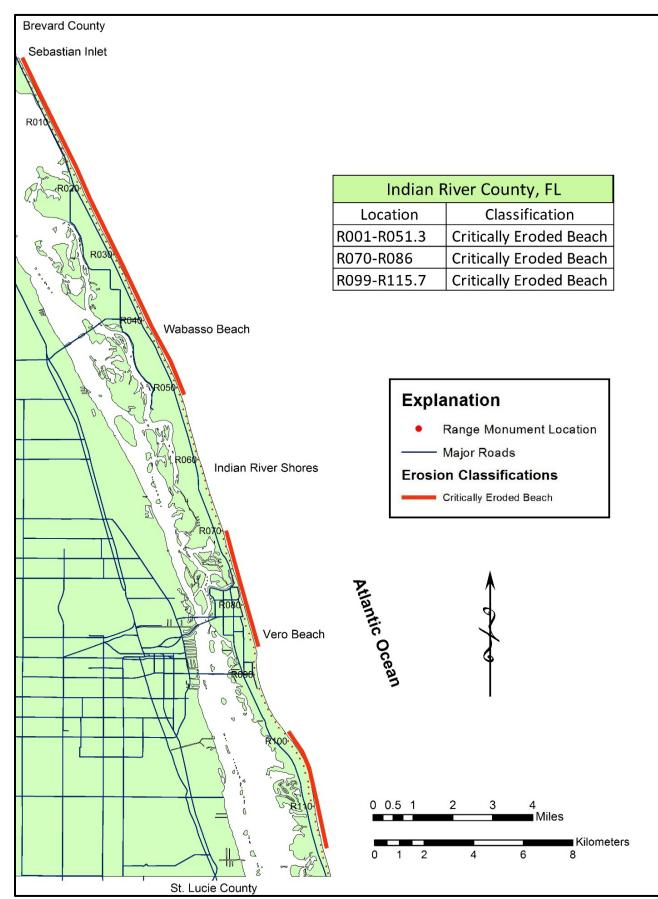
Figure 8. Critically eroded shoreline within Indian River County.
