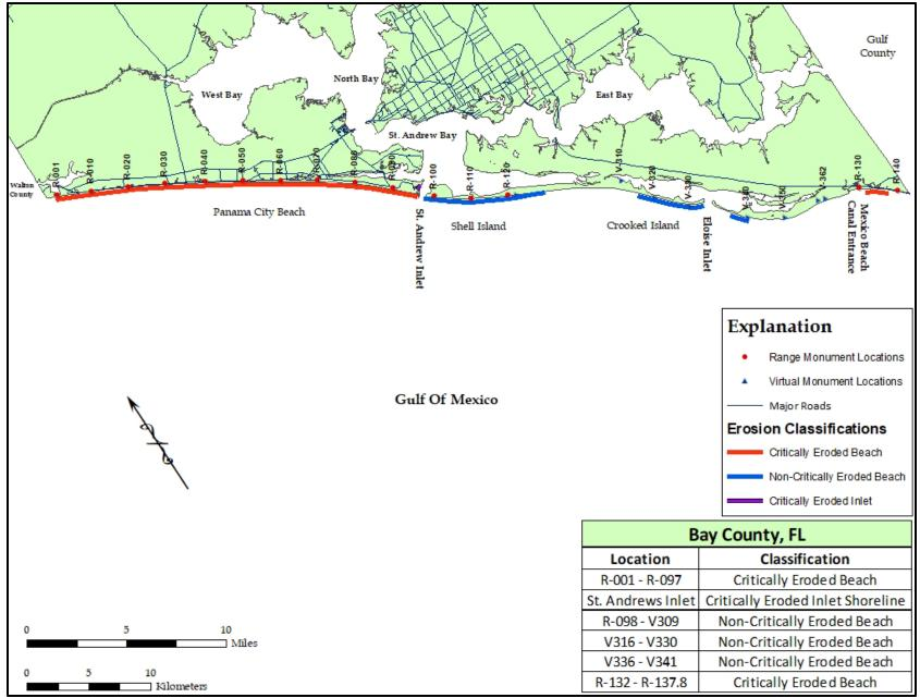
Figure 19. Critically eroded shoreline within Bay County.
