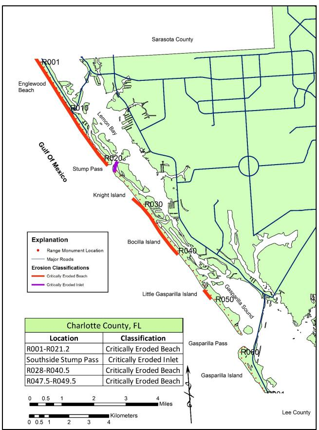
Figure 30. Critically eroded shoreline within Charlotte County.
