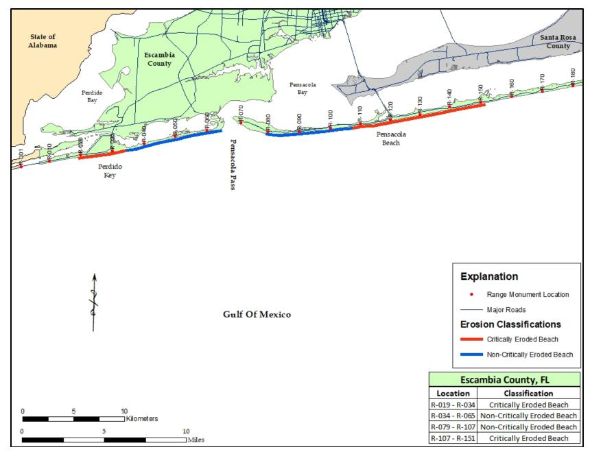
Figure 15. Critically eroded shoreline within Escambia County.
