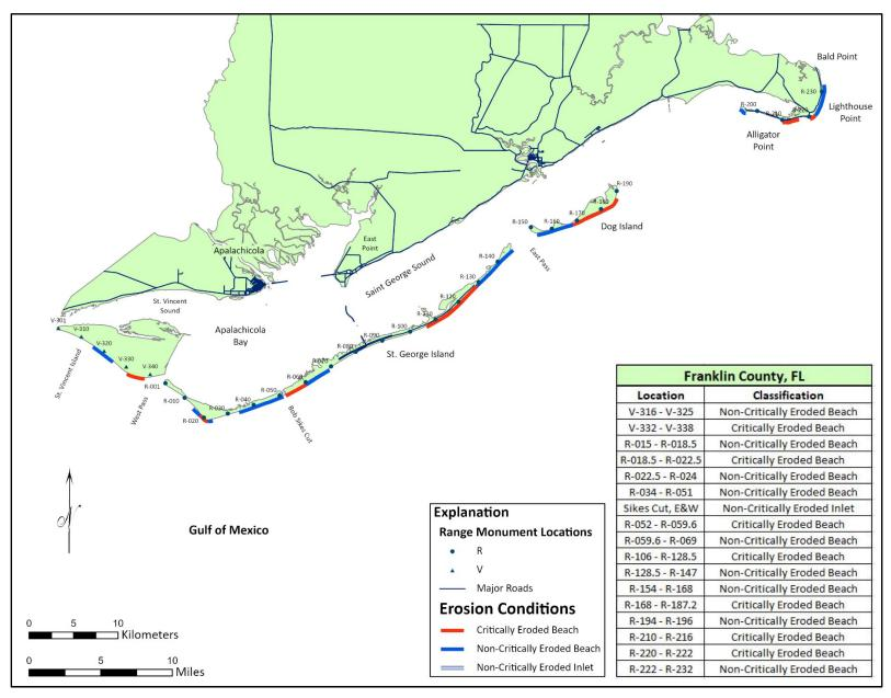
Figure 21. Critically eroded shoreline within Franklin County.
