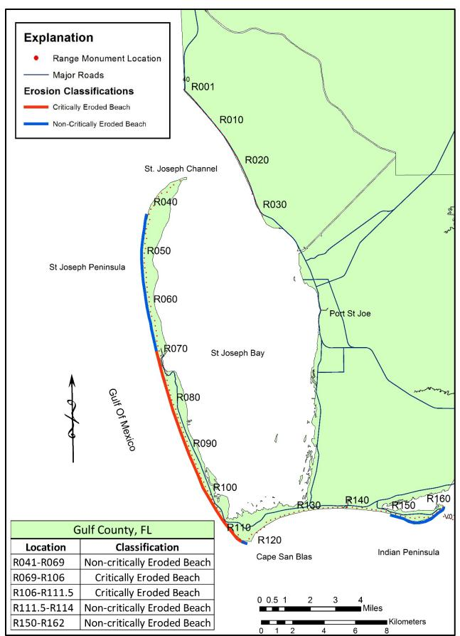
Figure 20. Critically eroded shoreline within Gulf County.
