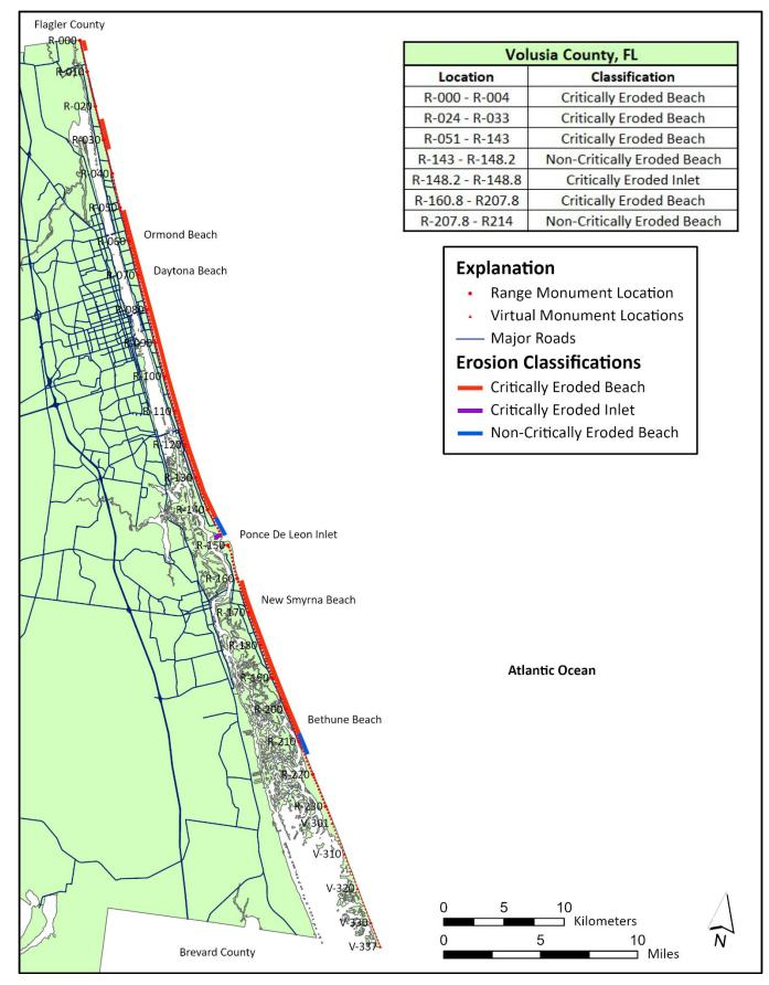
Figure 6. Critically eroded shoreline within Volusia County.
