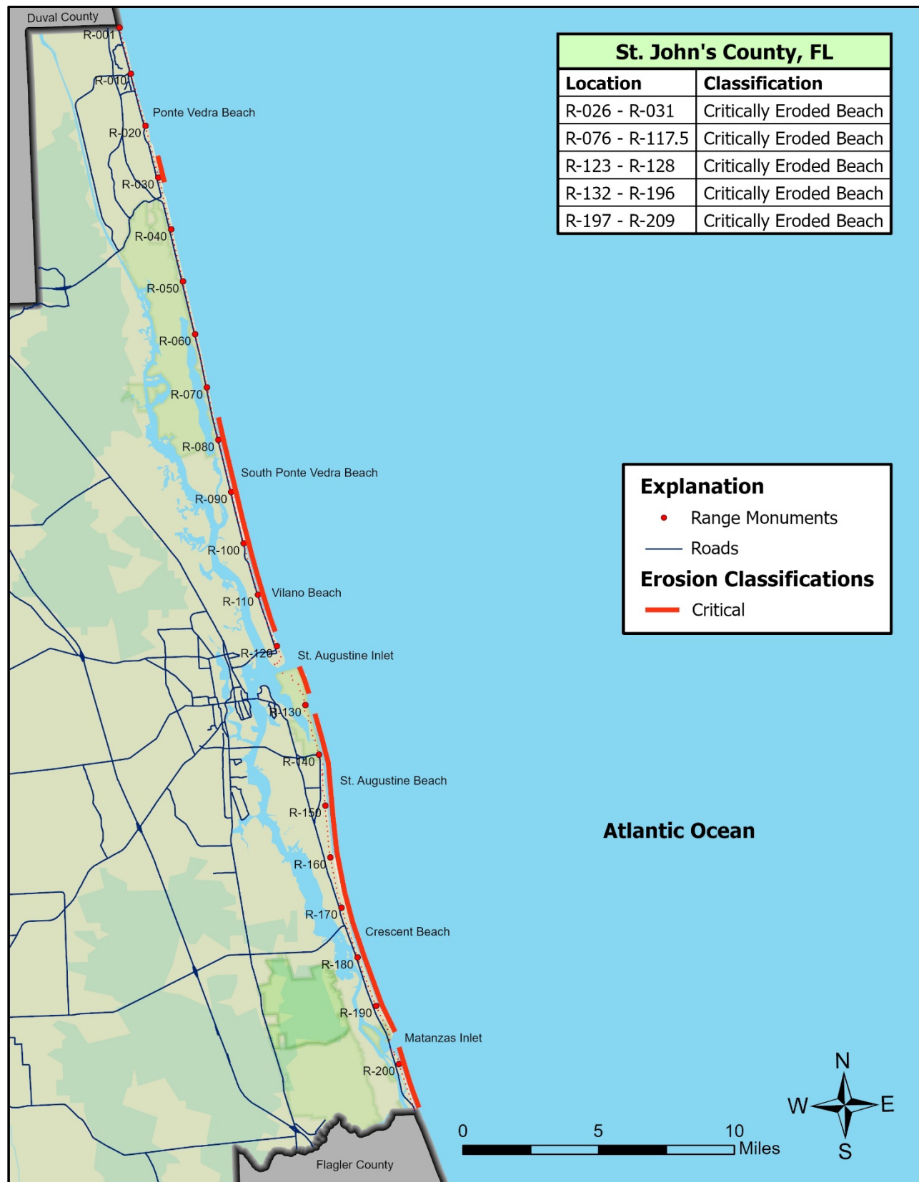
Figure 4. Critically eroded shoreline within St. Johns County.
