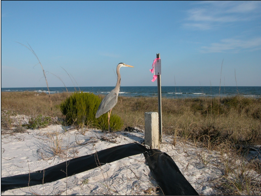
Figure 1. Range survey monument R-32 on Perdido Key in Escambia County, Fl.
