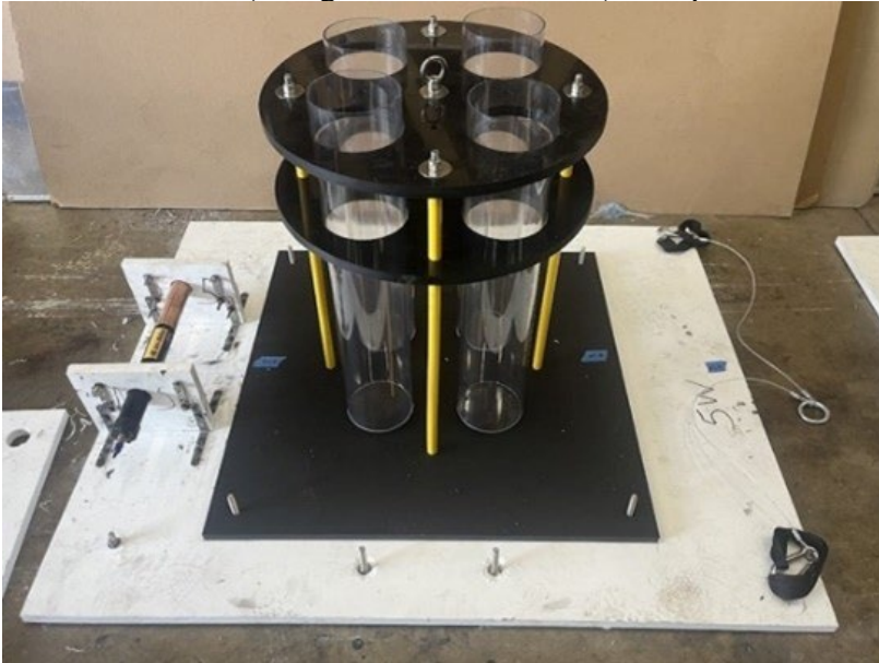
Figure 1. Constructed platform with ST-30 sediment trap and Aqua TROLL 600 sonde.
