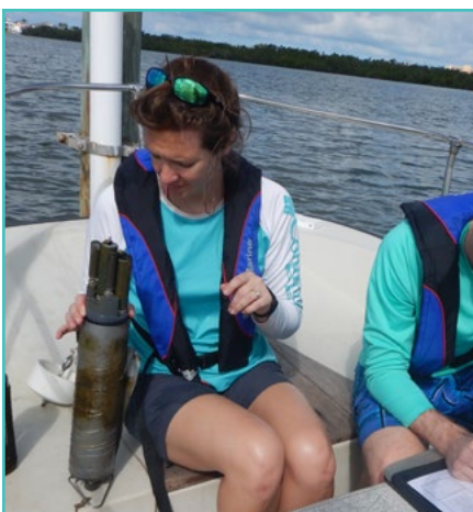
Estero Bay Aquatic Preserve water quality technician inspects a data sonde after deployment while a colleague records notes.
