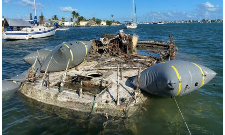
Marine debris removal in the Florida Keys using lift/float bags (Source: FWC)
