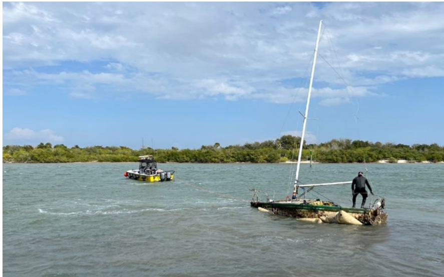
Derelict vessel removal utilizing a combination of methods: towing, float bags, and manual (diver) assistance (Source: FWC)
