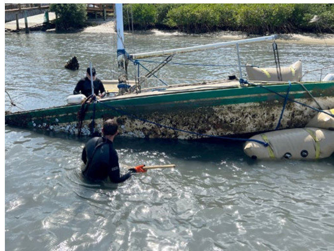
Manual assistance to derelict vessel removal via floating method (Source: FWC)
