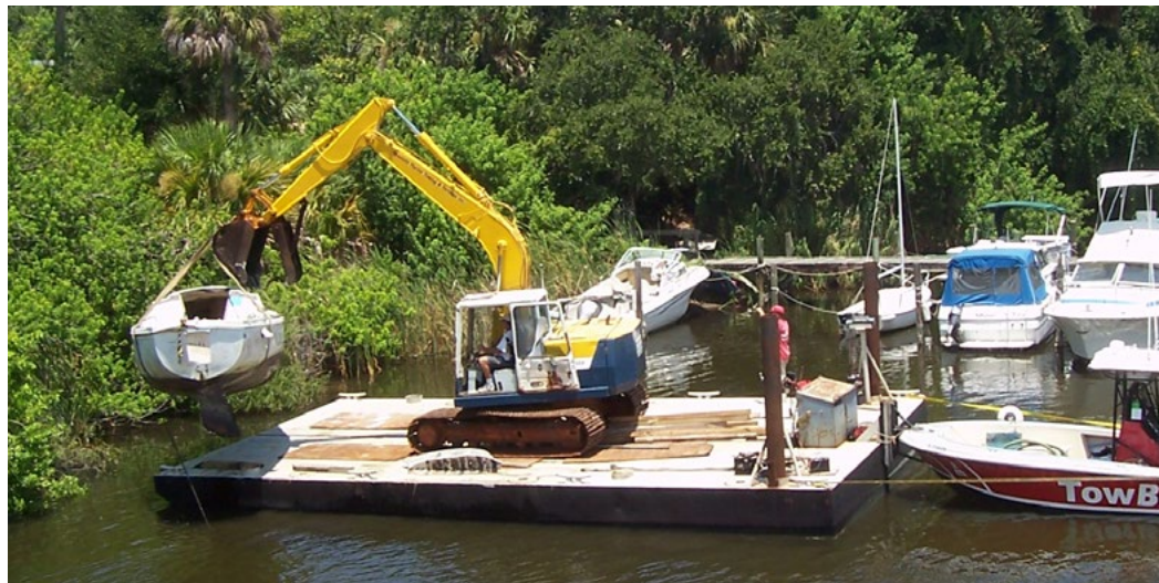
Barge-mounted excavator performing lifting technique to remove a derelict vessel in Northeast Florida (Source: FWC)
