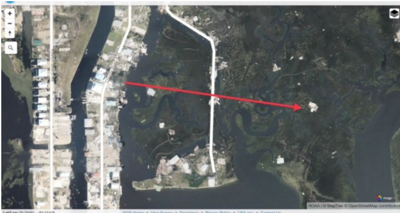
Figure 17. Keaton Beach dwellings carried into the marsh by the storm surge (NOAA photo).
