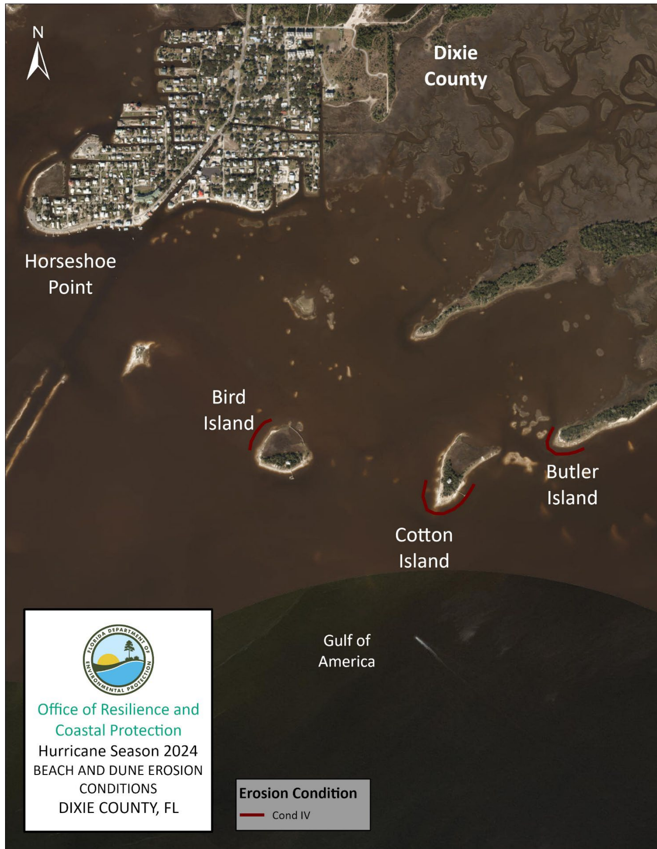
Figure 29. Northern Dixie County beach and dune erosion conditions from Hurricane Helene.
