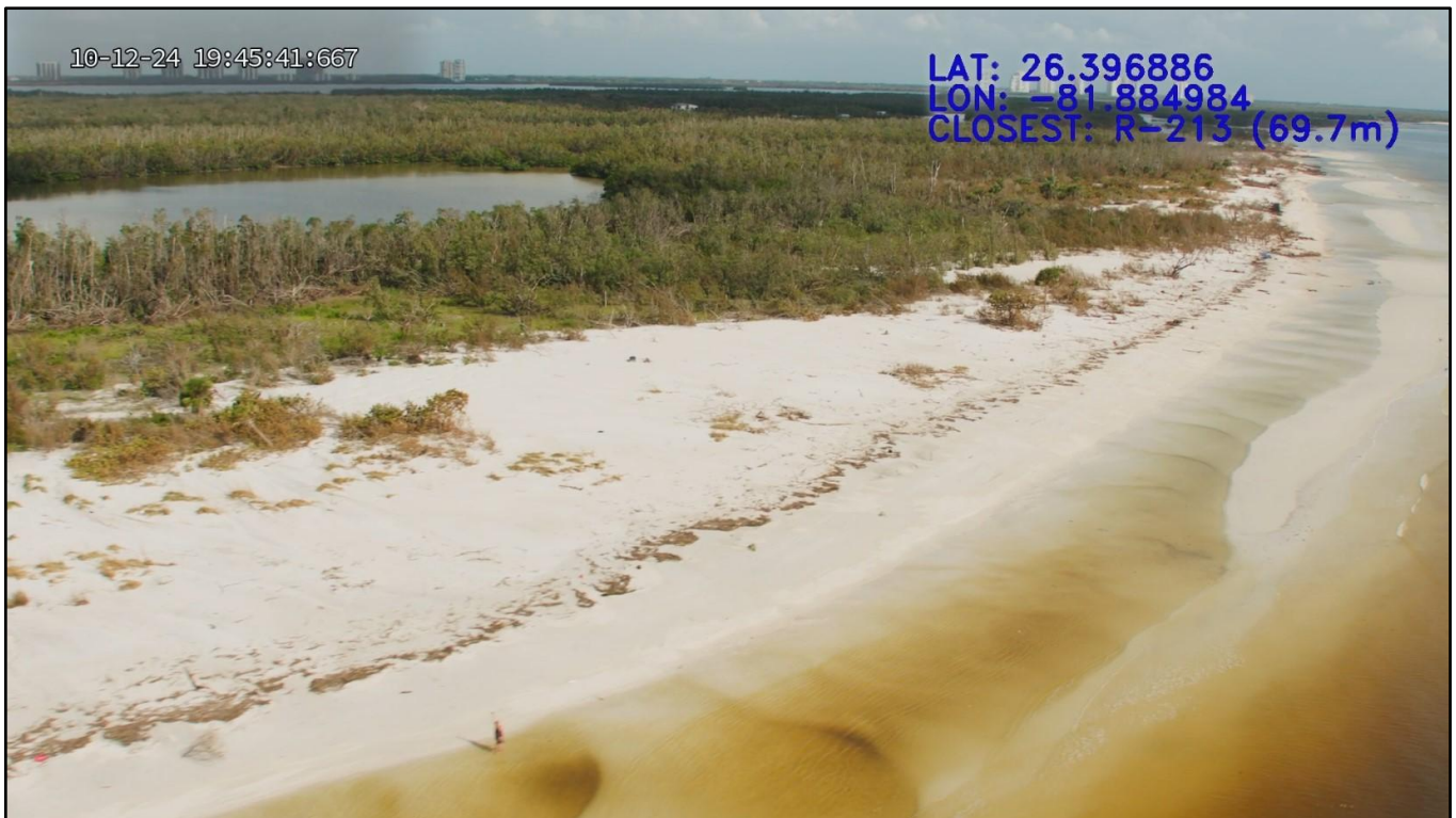
Figure 137. Nearshore storm-built sandbar with major beach and dune erosion (condition IV) due to Helene and Milton at Lover's Key State Park near R-213.
