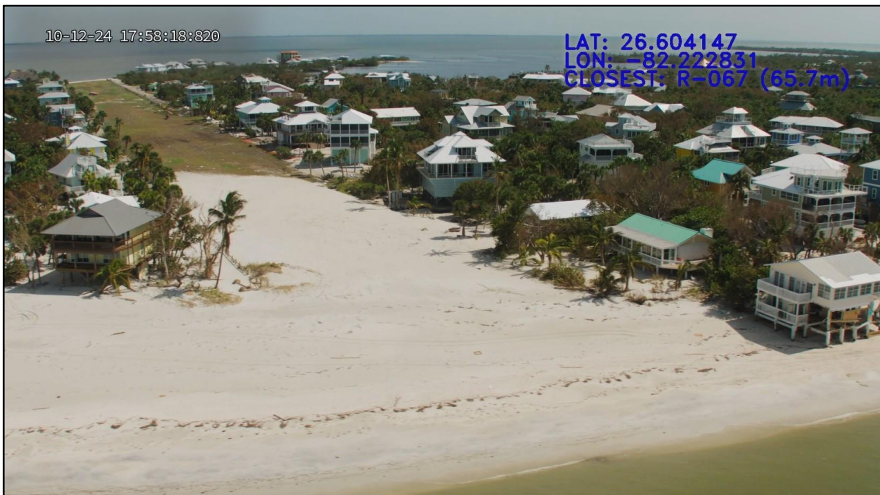
Figure 129. Major beach and dune erosion (condition IV) and storm surge overwash on an airport runway on North Captiva Island near R-67.
