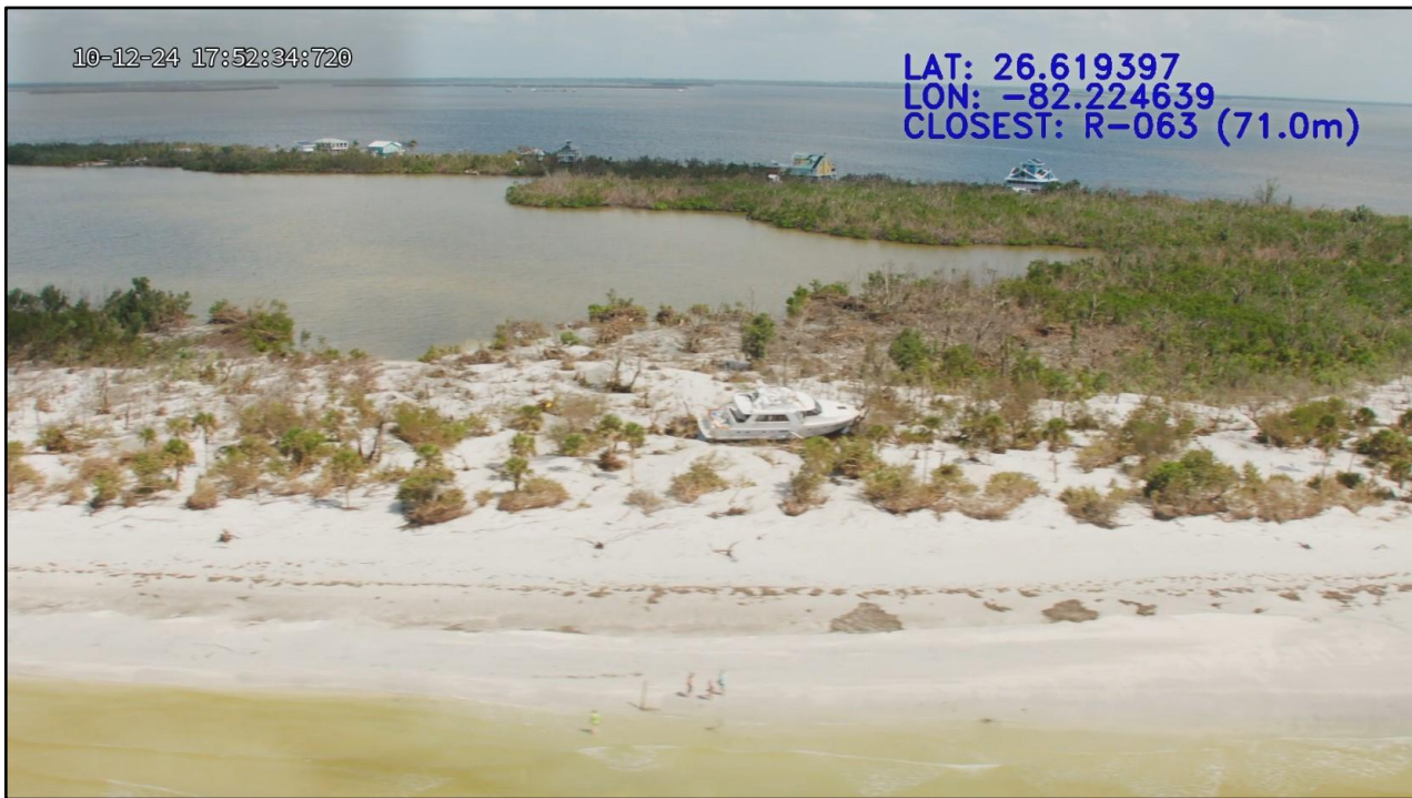
Figure 128. Major beach and dune erosion (condition IV) and stranded boat on Cayo Costa near R-63.
