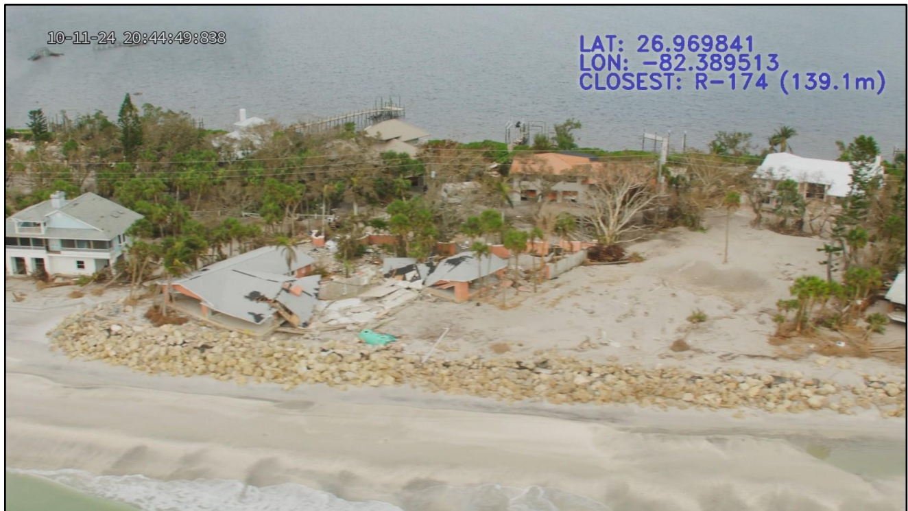
Figure 105. Single-family dwelling destroyed and major revetment damage by Milton on Manasota Key, R-173.
