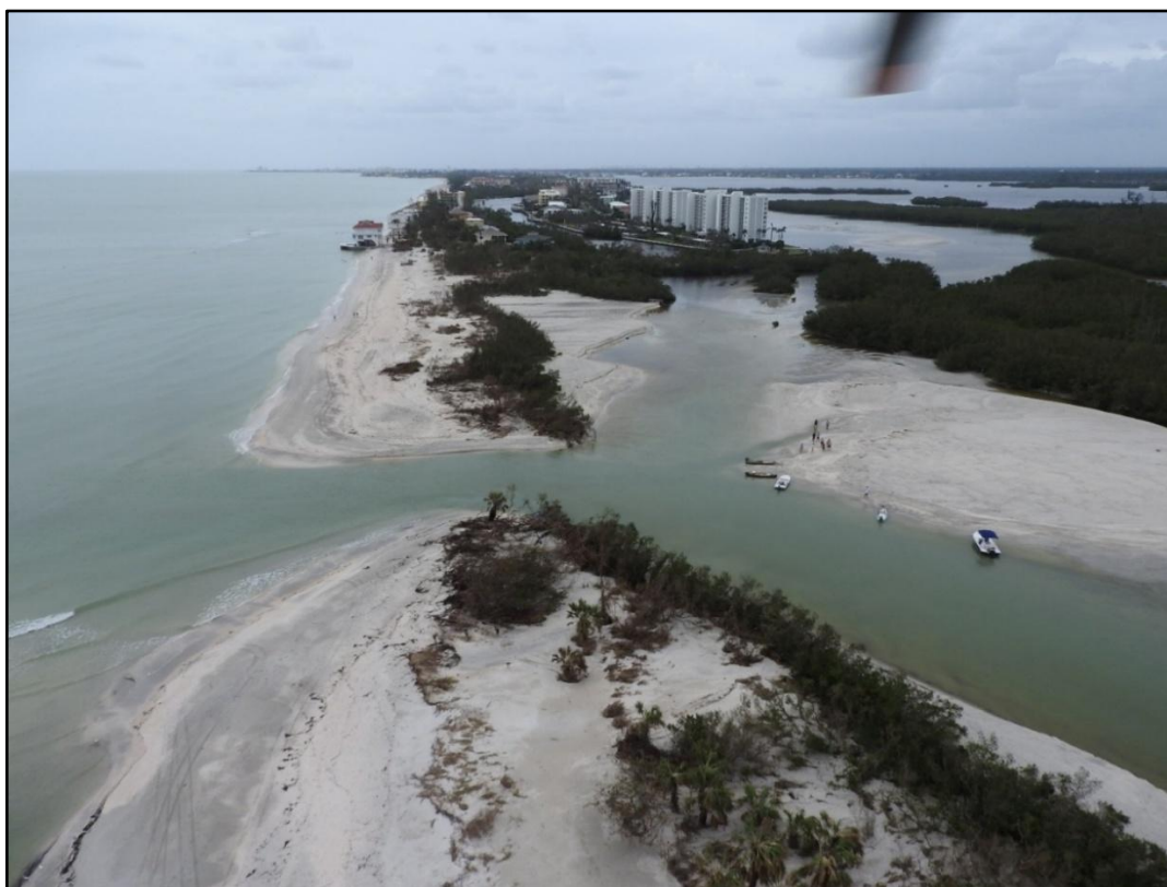
Figure 67. Enlarged breach near R-78 at Midnight Pass due to Milton. Photo taken on October 11, 2024.
