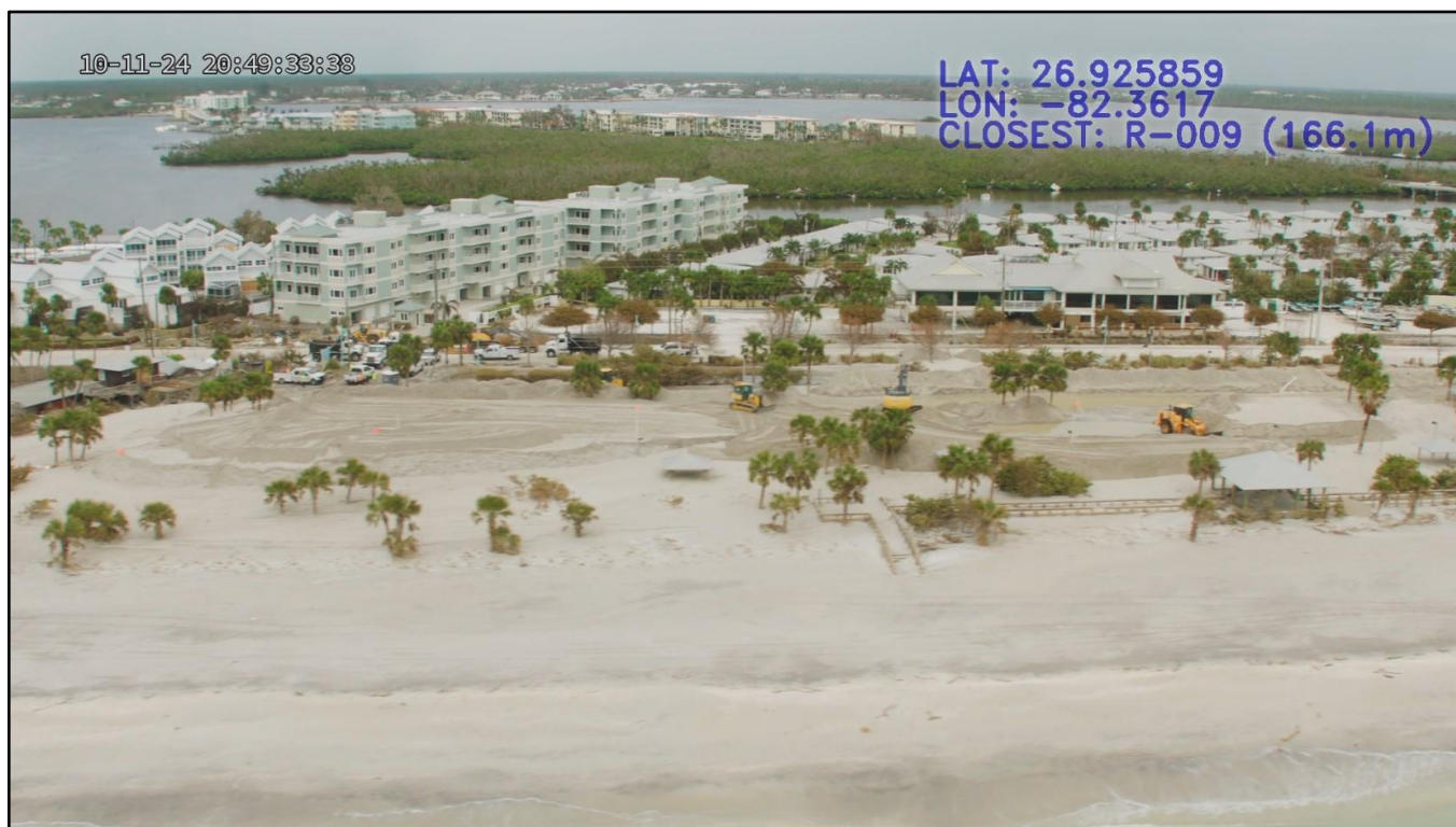
Figure 109. Major beach erosion and sand overwash deposited in parking lot at Englewood Beach Park due to Helene and Milton near R-9.
