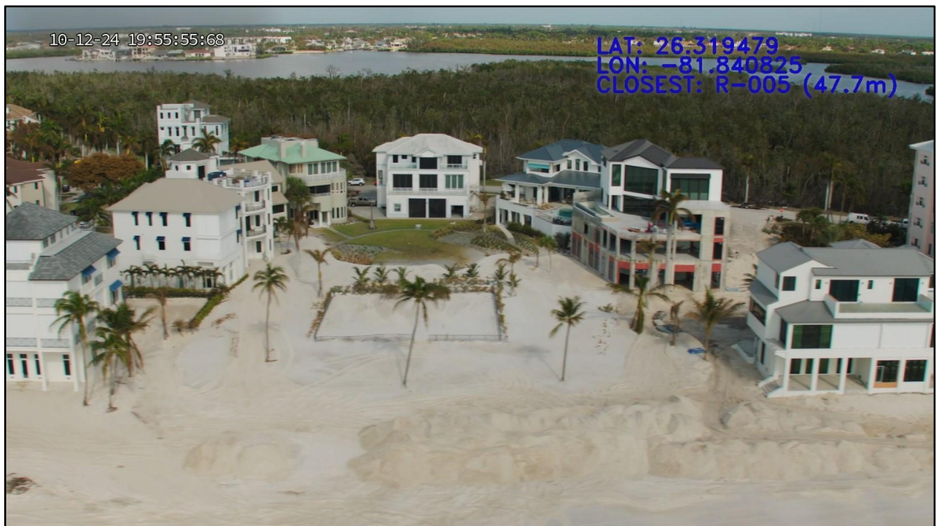
Figure 146. Major beach and dune erosion (condition IV) from Helene and Milton's storm surge which filled the pool with overwash sand at Barefoot Beach near R-5.
