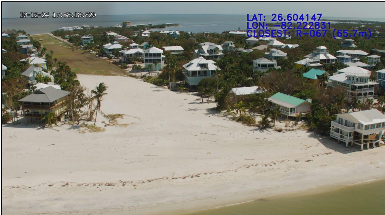
Figure 129. Major beach and dune erosion (condition IV) and storm surge overwash on an airport runway on North Captiva Island near R-67.
