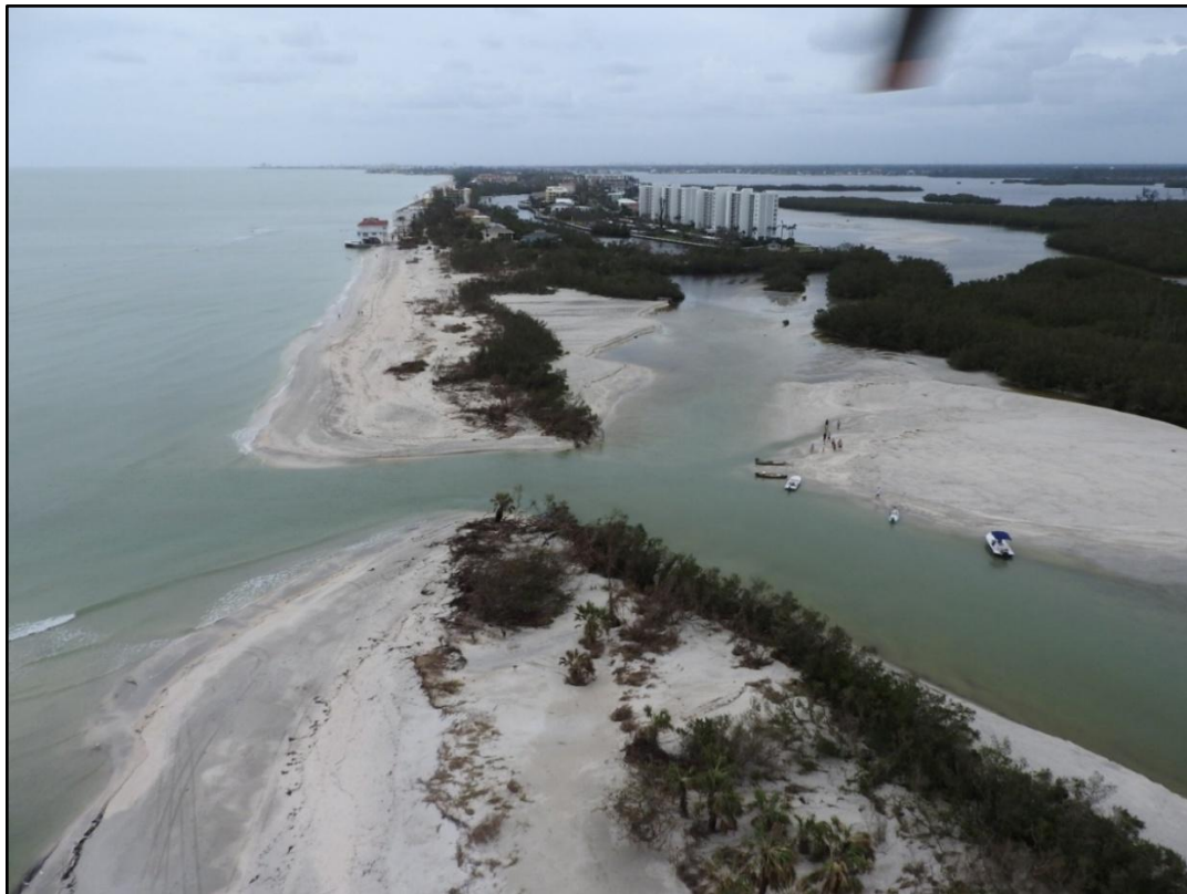
Figure 67. Enlarged breach near R-78 at Midnight Pass due to Milton. Photo taken on October 11, 2024.
