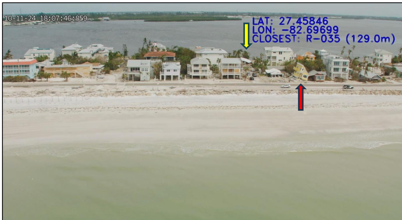
Figure 45. Major beach and dune erosion (condition IV) due to Helene and Milton on Anna Maria Island (R-35). Note the home toppled due to wind from Milton (red arrow) and the home impacted by Helene’s storm surge that was carried into the middle of 12th Street South (yellow arrow).
