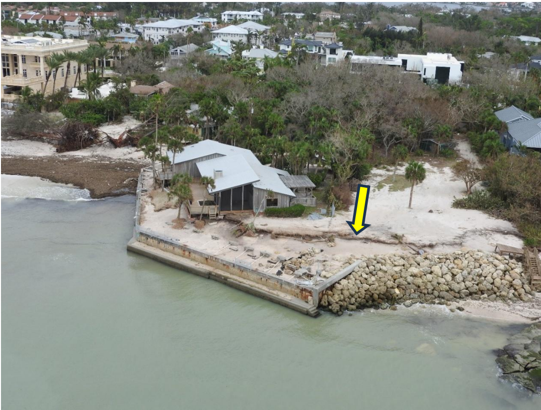
Figure 62. Major erosion (condition IV) with an escarpment at +8 to +9 feet on Siesta Key at Point of Rocks near R-62.
