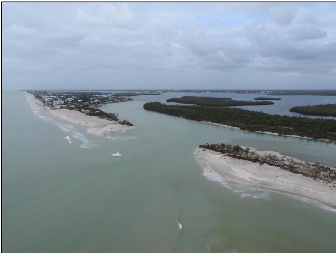
Figure 110. A major breach on Manasota Key in Stump Pass State Park by Milton (R-17).
