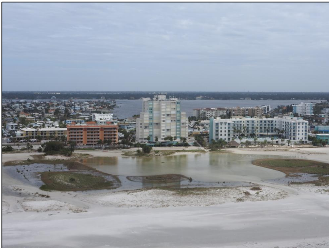
Figure 17. Major beach and dune erosion (condition IV) following Helene and Milton on Treasure Island (R-131).
