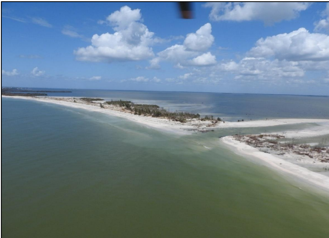
Figure 130. A breach to North Captiva Island and substantial overwash due to Helene and Milton at R-79.
