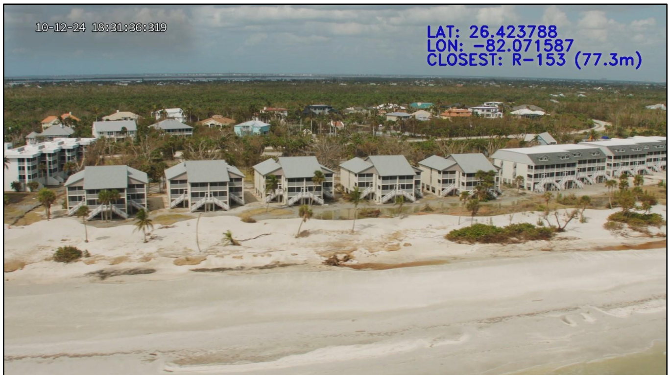
Figure 133. Major beach and dune erosion (condition IV) due to Helene and Milton on Sanibel Island near R-153.
