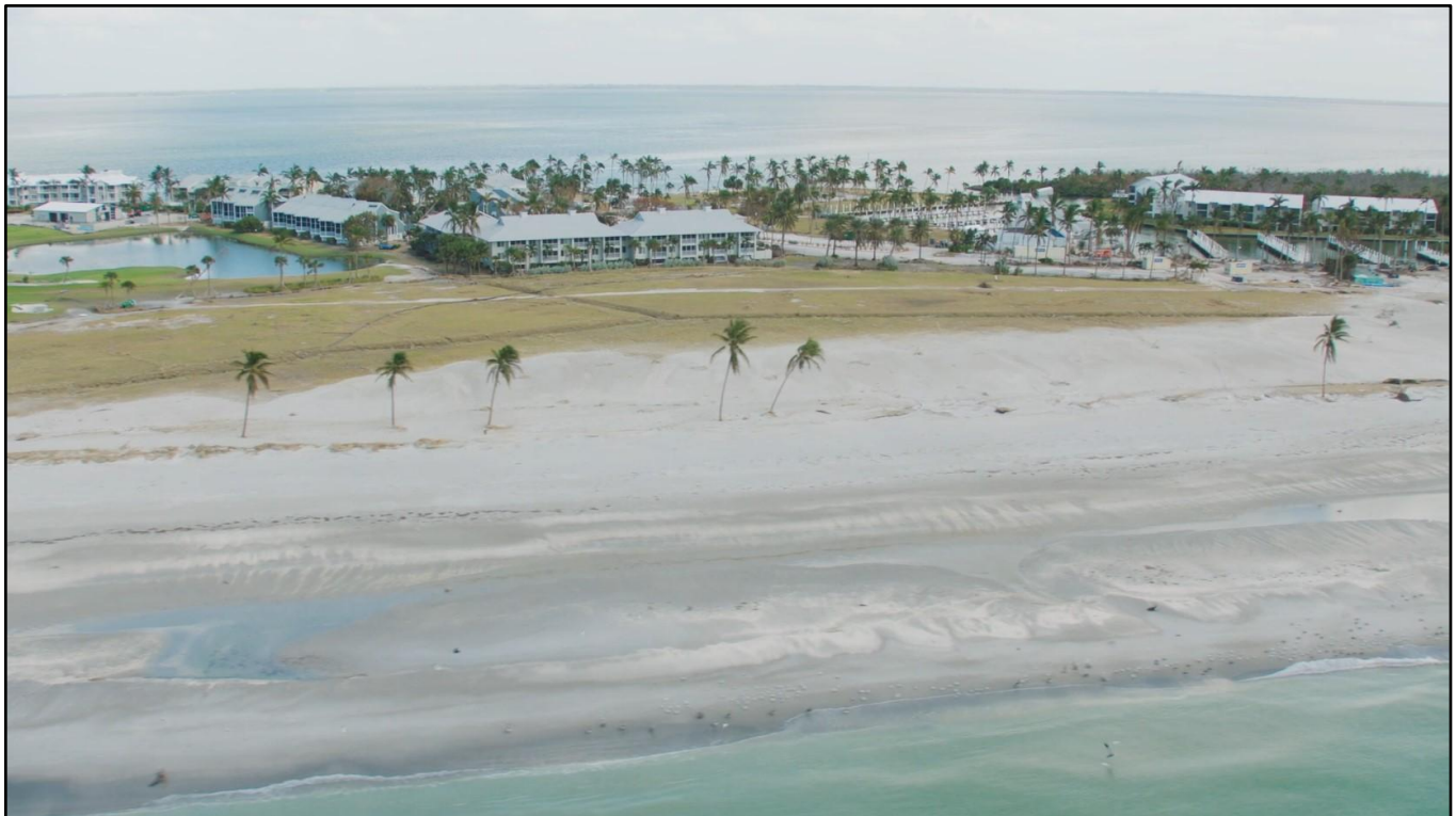
Figure 132. Major beach and dune erosion (condition IV) due to Helene and Milton at South Seas Plantation on Captiva Island near R-85.
