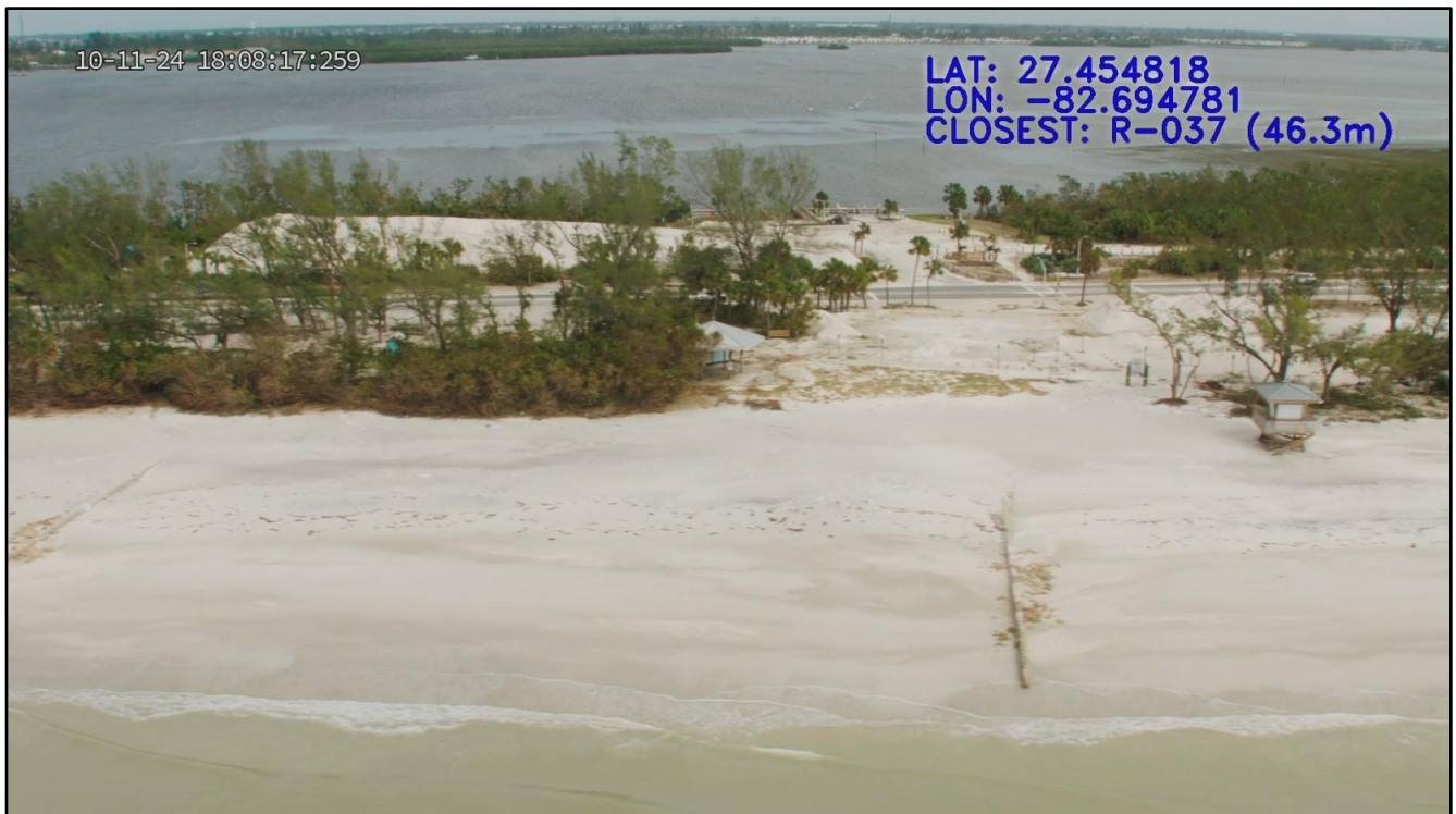
Figure 31. Major beach and dune erosion (condition IV) and stock-piled sand after Helene and Milton, at Coquina Beach, Anna Maria Island near R-37.
