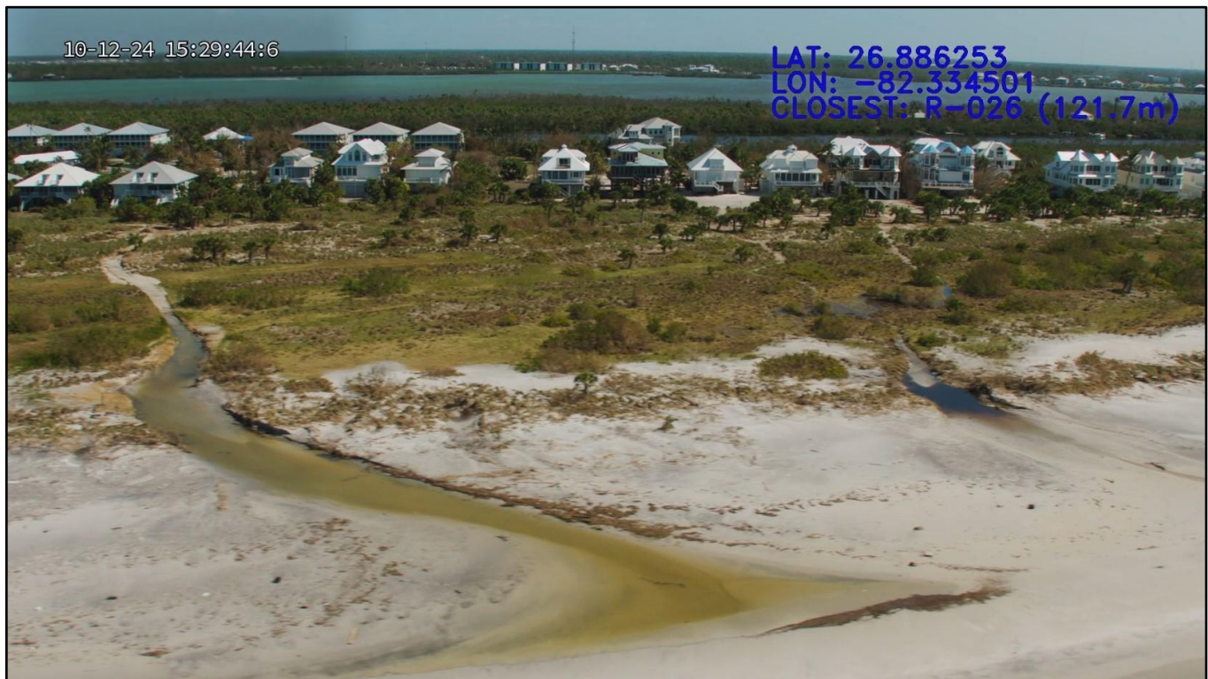
Figure 111. Storm surge discharge gullies at the Palm Island development on Don Pedro Island (R-26).
