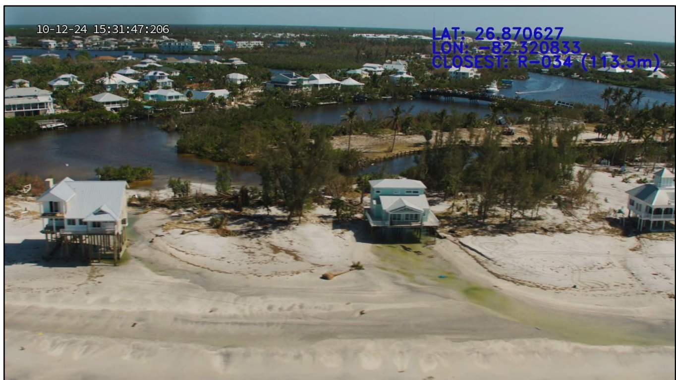
Figure 112. Storm surge discharge gullies on Don Pedro Island near R-34.
