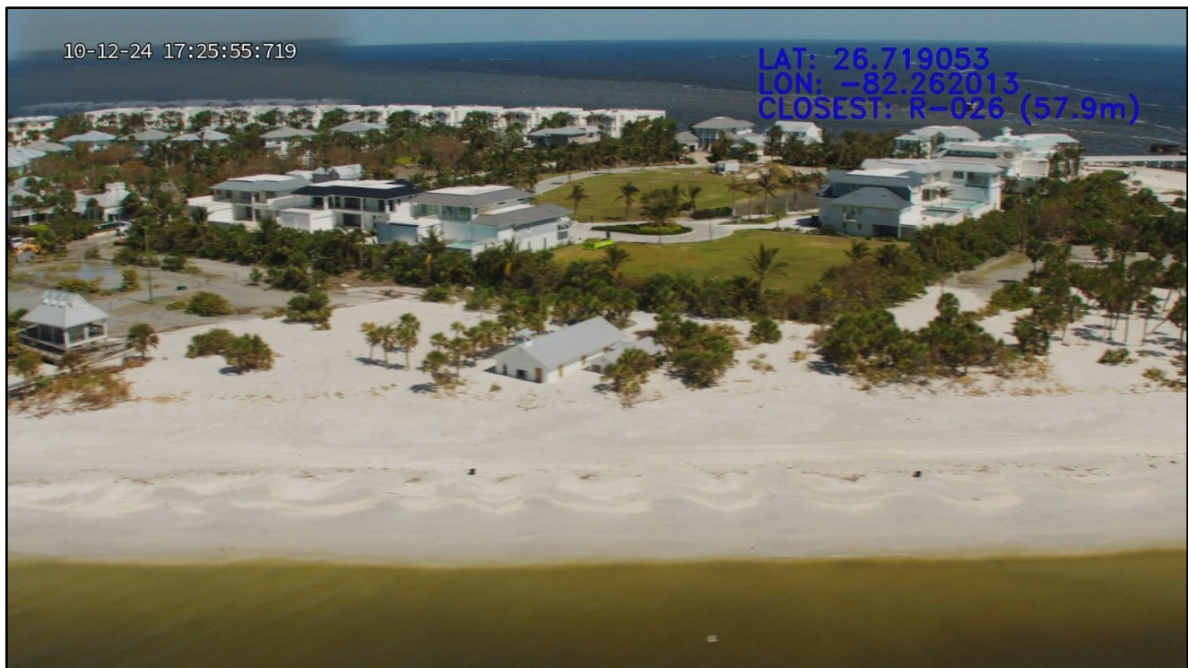
Figure 127. Major beach and dune erosion and storm surge overwash due to Helene and Milton at Gasparilla Island State Park and at a historic church building at R-26.
