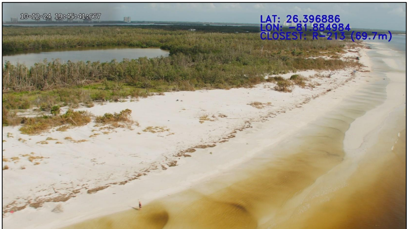
Figure 137. Nearshore storm-built sandbar with major beach and dune erosion (condition IV) due to Helene and Milton at Lover's Key State Park near R-213.
