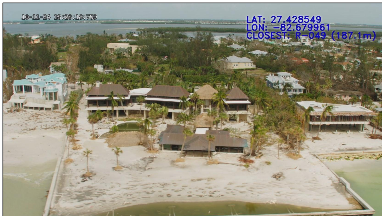
Figure 48. First floor flooding damage, seawall damage and major erosion (condition IV) following Helene and Milton on northern Longboat Key near R-49.
