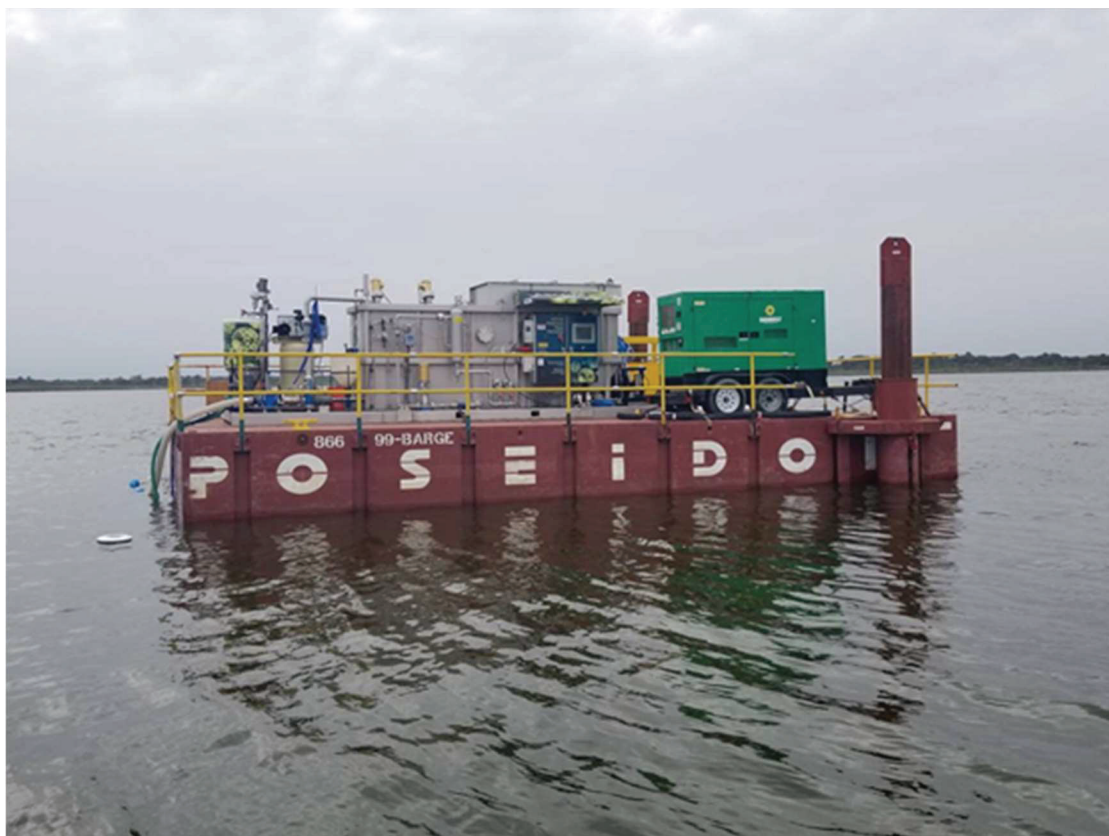
Barge positioned at Barge Station 1 south of Bird Island. HFT algae harvester (silver) and 56 kW generator with secondary containment (green) are secured to the deck with chain and ratchet strap binders. Spuds are lowered into the lakebed to hold the barge in place.
