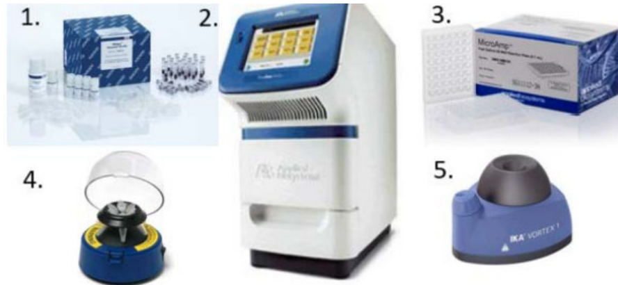
(a) qPCR instrument and accessories used at UCF Lab. which include 1). DNeasy PowerSoil kit, 2). Applied Biosystem StepOne qPCR System, 3). PCR 48-well plate, 4). Centrifuge, and 5). Vortex mixer
