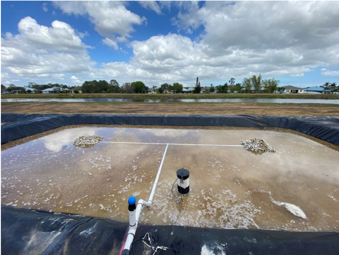
Figure 3-9: Test run at cell #4 (CPS) with the stilling well in the middle.
