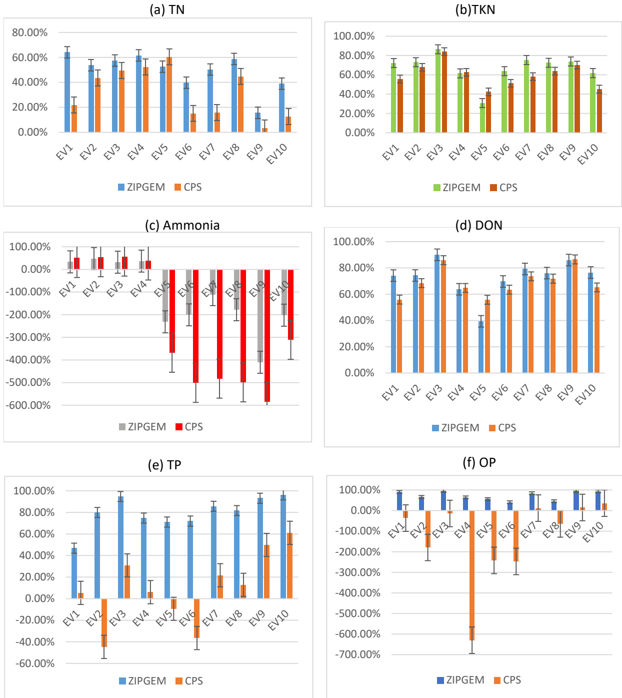
Figure 4-6: The removal efficiency of (a) TN, (b) TKN, (c) Ammonia, (d) DON, (e) TP, and (f) OP by ZIPGEM and CPS
