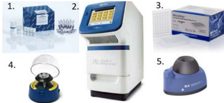
(a) qPCR instrument and accessories used at UCF Lab. which include 1). DNeasy PowerSoil kit, 2). Applied Biosystem StepOne qPCR System, 3). PCR 48-well plate, 4). Centrifuge, and 5). Vortex mixer
