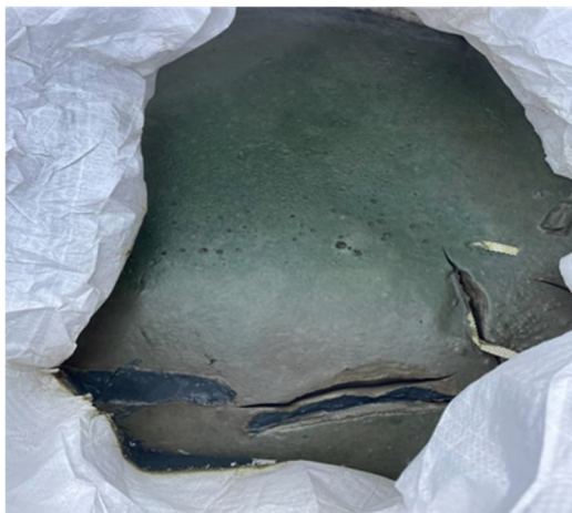
Recovered algae biomass being dewatered in a dewatering mesh bag.
