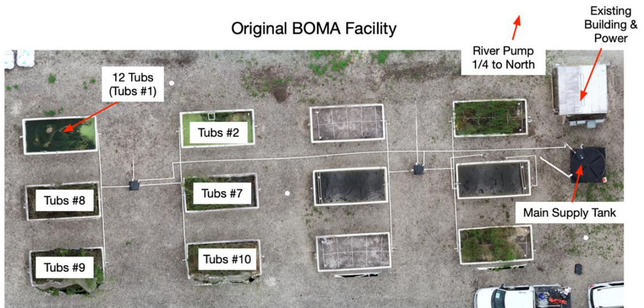
Figure 4. Layout of the site showing the main supply tank, the storage building with the power supply, and the tubs containing the vegetation.
