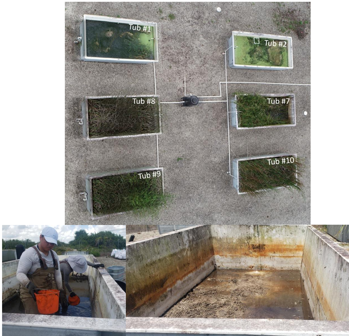
Figure 15. Top: Vegetative state of the tubs prior to being cleaned (07/02/2021). Photo taken with an aerial drone (DJI™ phantom 4 Pro). Bottom left: cleanup of the phytodetritus and sediment. Bottom right: tub after being cleaned.
