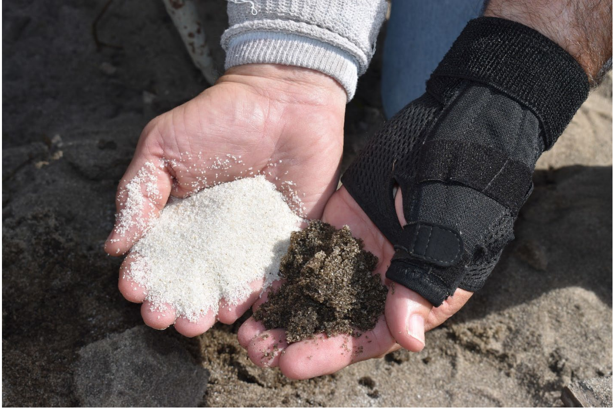
Figure 6. Comparison of clean sand and Schmutzdecke removed during maintenance of sand filter (3/23/22)
