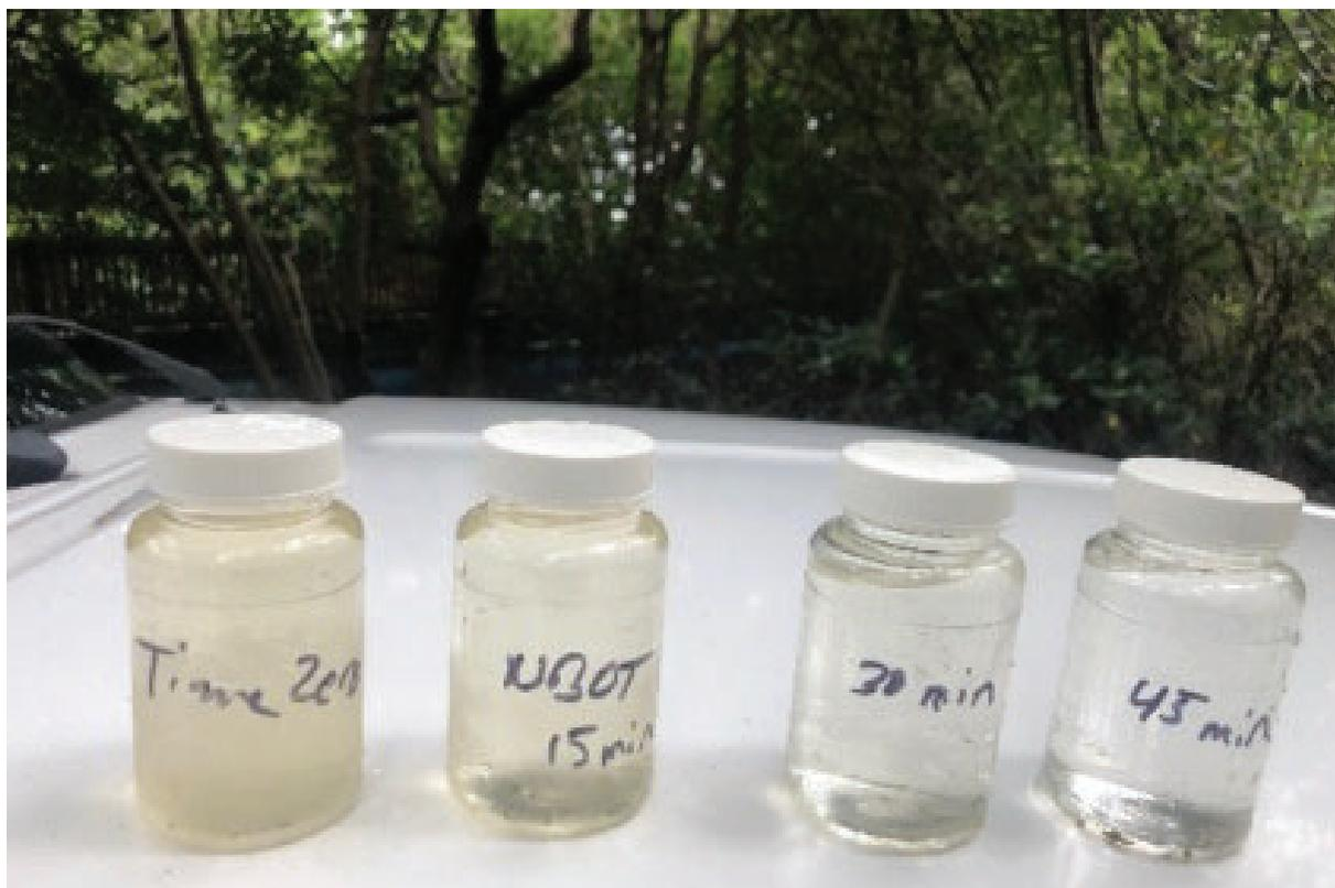
**Photo 1.** Photo of water samples collected in recirculating tank test from NBOT 2 on September 2, 2021 showing increased water clarity over time from time zero to 45 minutes.
