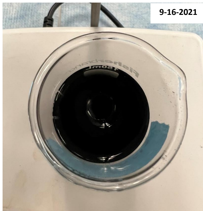
Figure 36: Vortex forming during the mixing of adsorbent and solution.
