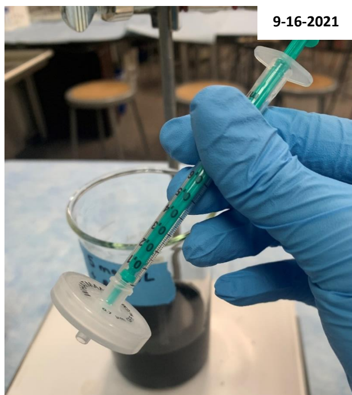
Figure 37: Syringe and syringe filter used to filter the adsorbent from the solution.
