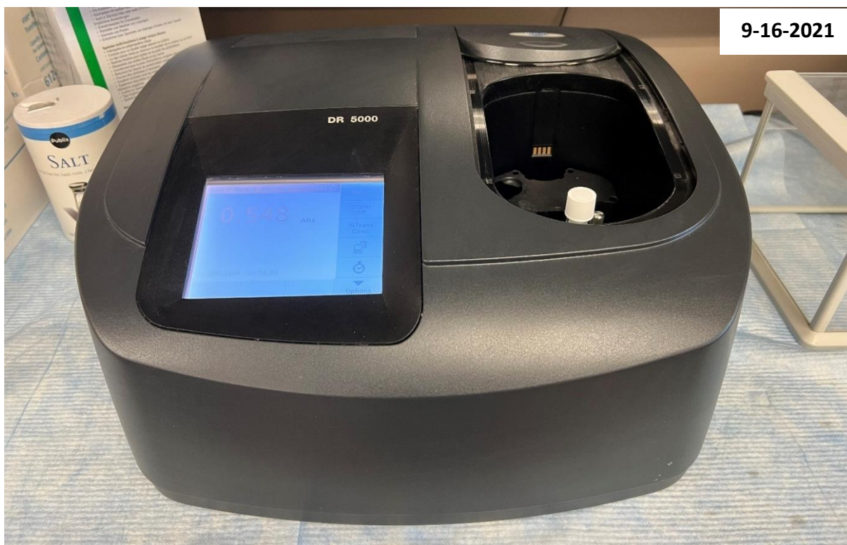
Figure 34: Absorbance being measured in the DR 5000 spectrophotometer.
