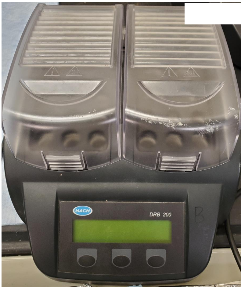
Figure 92: Hach DRB 200 Reactor.
