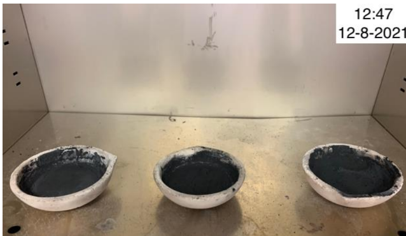
Figure 79: Mixture of MA and precursor in oven.
