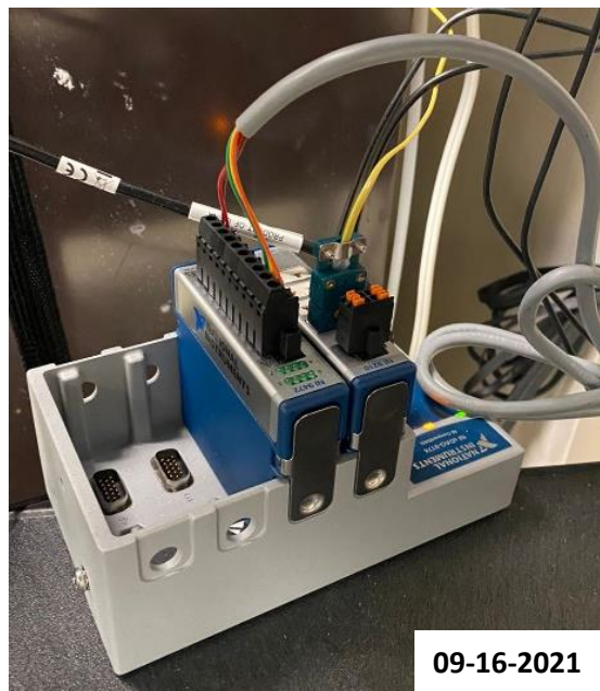
Figure 17: Data acquisition chassis made by National Instruments.
