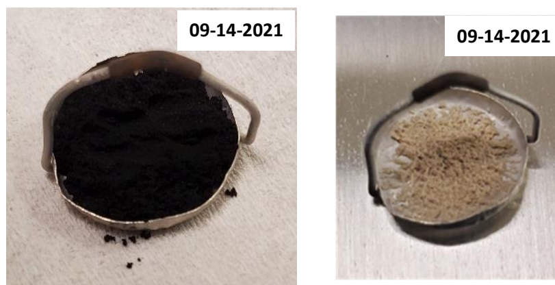
Figure 26: TGA sample holders before and after testing. Left: Commercial activated carbon before heating. Right: Residual ash from commercial activated carbon after heating.
