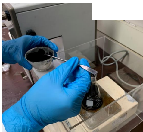
Figure 27: Acid treatment procedures. Top row: (left) HCl solution, and (right) student researcher preparing acid solutions. Bottom row: (left) student researcher transferring the activated carbon to acid solution, and (right) stirring the acid solution and activated carbon.
