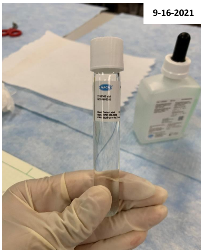
Figure 29: Reactive Phosphorus Test 'N Tube Vial with no sample added.
