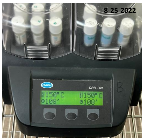
Figure 95: COD test vials being heated in Hach DRB 200 Reactor.
