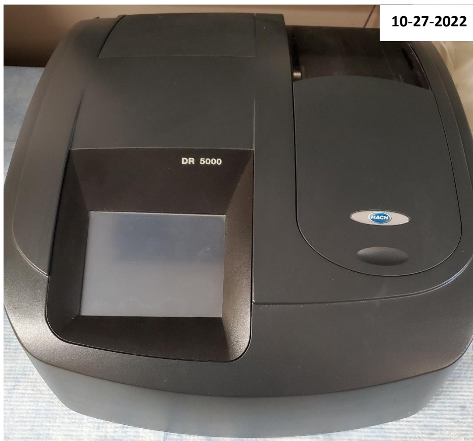
Figure 93: Hach DR 5000 UV-Vis Laboratory Spectrophotometer.
