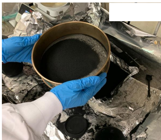
Figure 22: Left: Ground AC on sieve No. 100. Right: Student researcher sieving the carbon.
