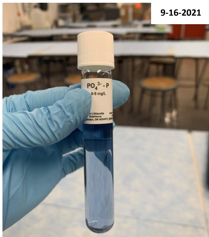
Figure 31: Reactive Phosphorus Test 'N Tube Vial after the sample and PhosVer 3 Phosphate Powder Pillow packet has been added to the test tube.
