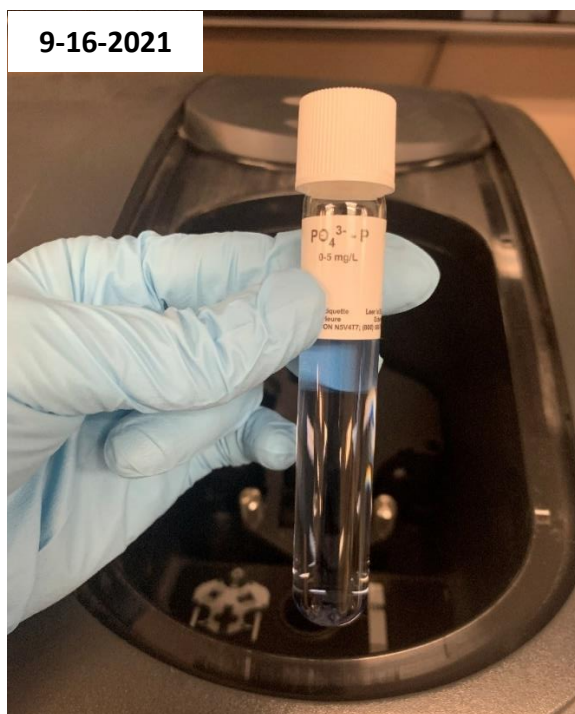
Figure 30: Spectrophotometer being zeroed out with just the Reactive Phosphorus Test 'N Tube Vial and 5 mL of sample.
