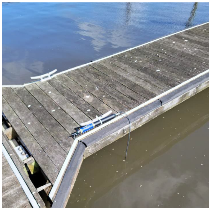
Figure 8: Treatment area In-Situ water quality monitoring sensor mounted on D Dock.
