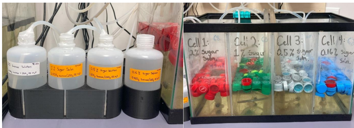
Figure 11. Images of flow through carbon concentrations (%) dosed into the flow through bioreactor for different carbon to nitrogen ratios.
