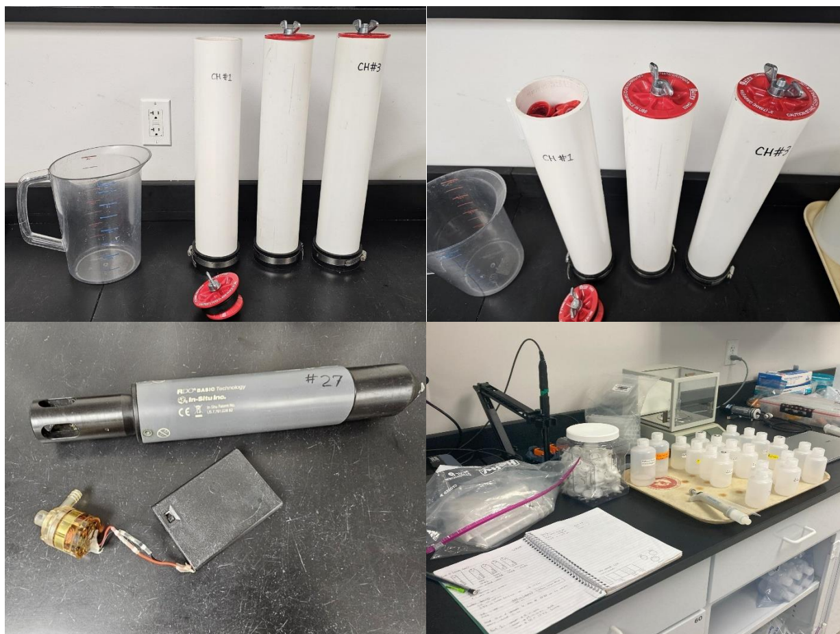
Figure 7. Images captured of batch bioreactor experiment A) Chambers, B) Chamber #1 showing packed bottle caps, C) The DO Logger and mechanical stirrer used inside the chambers during the experiment, and D) the set-up of the bottles to take samples and dose correct C:N ratios of carbon.
