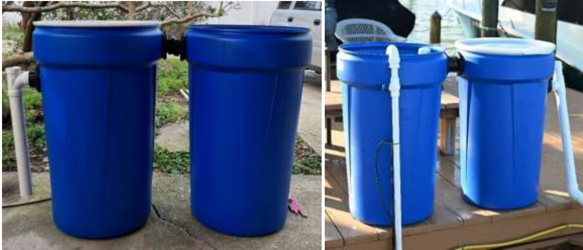
Figure 20: Image of the field demonstration of the modular system. The first image was taken during the build. The second image is the system as initially installed. Each module has a 55 gallon (208 liter) capacity. The pumping rate is 75 gallons/hour (300 l/hr). The image on the left shows the initial dry test fit of the system components, and on the right is the first iteration of the demonstration system as initially installed.
