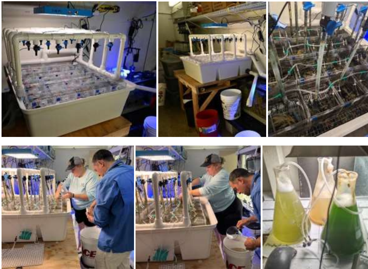
Figure 7: Laboratory grow out system for testing cultivation of sponges. The system consists of 20 two-liter cubes in a water bath. The water bath maintained a consistent temperature and provided an area for biofilter media. Additional breakdown of excess nutrients occurred in a system sump containing additional biofilter media. Water was supplied to each cube through a rate controlled system. When sponges were added, all effort was taken to ensure they remained immersed in water, and sufficient time was given for them to acclimate to lab conditions (temperature, salinity, pH). The final image shows three of the four foods (l - r): phytoplankton, marine broth and phytoplankton + marine broth.
