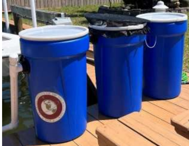
Figure 22: Field system with the dosing module installed.
