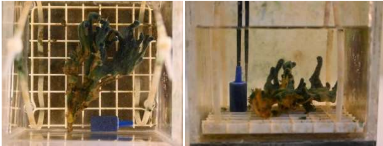
Figure 11: Measuring the sponges using the 2D approach. This method uses an object of known size (an air stone) and two images, one from above and one from the side, to measure changes in size over time. It has proven to be a simple, reproducible and robust method for measuring sponge growth. Because of the modifications to the lab system, sponges are removed from their growing cubes and measured without ever being removed from the water.
