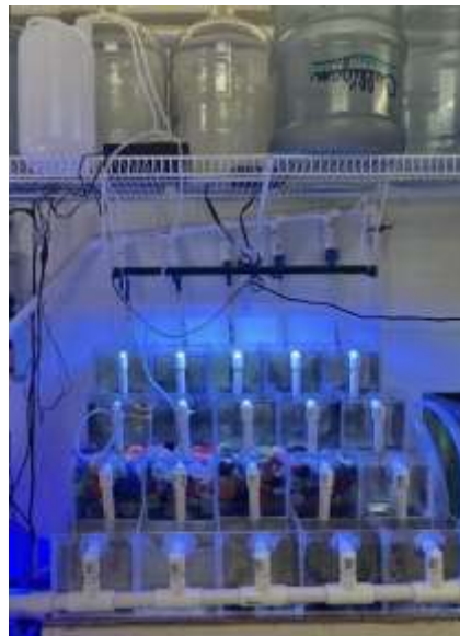
Figure 13: Lab setup after sugar dosing system was added. The white bottle in the upper left holds the sugar solution. Inside the black box are peristaltic pumps, adding microdoses of the sugar solution. The dosing is maintained at a C/N molar ratio of 9. The sugar is being supplied to the two cubes on the left through flexible silicone tubing.
