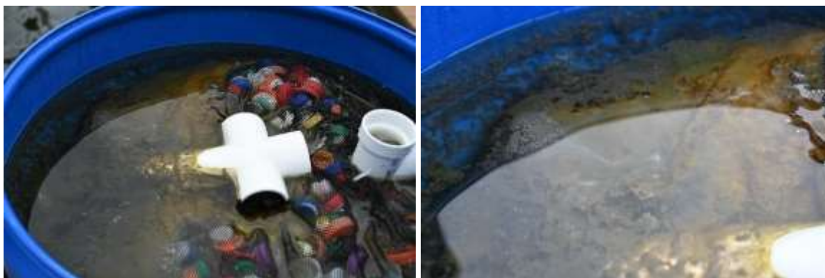
Figure 24: Growth of biofilms in the modules after sugar was added. The biofilm has become thick, opaque and cohesive.
