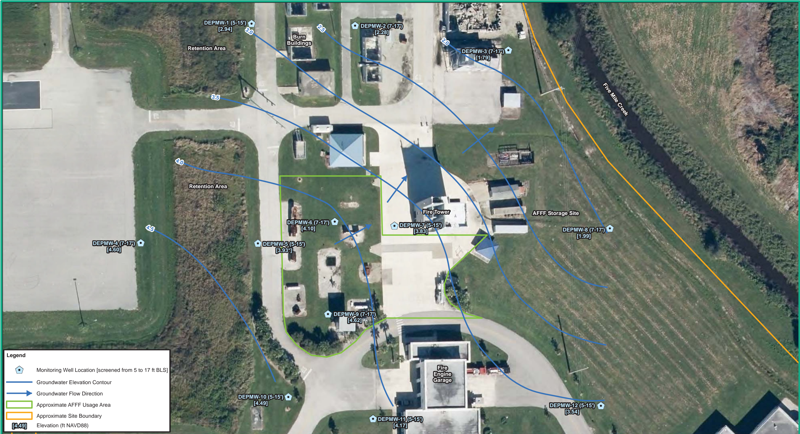
Figure 6 Groundwater Elevation Contour Map from 5 to 17 ft BLS Indian River State College 4600 Kirby Loop Road Fort Pierce, St. Lucie County, Florida
